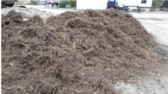
Photo #13: Mulch mix- Blended 40% by volume into bank run import fill material. Placed inside membrane.
