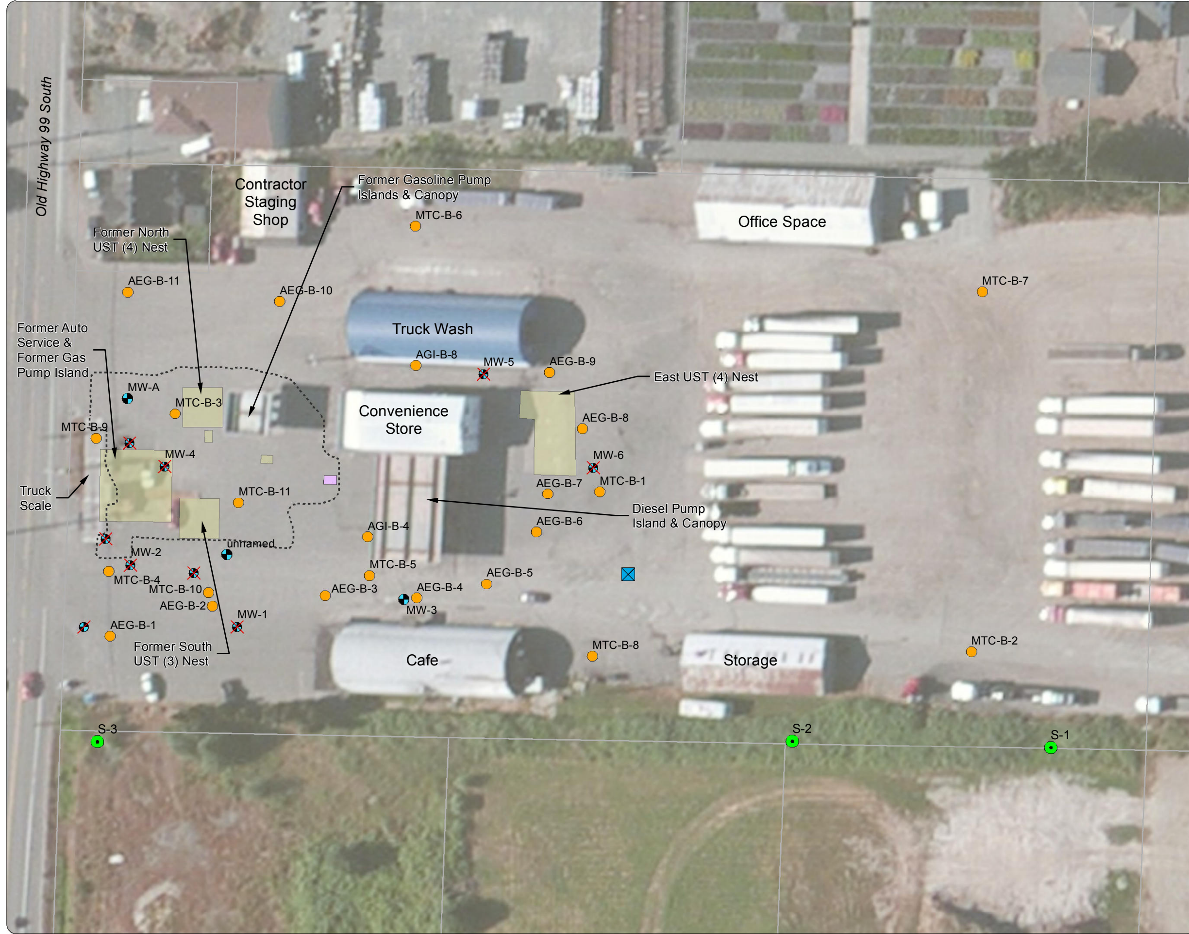
Figure 2-1 Pre-Remedial Action Site Features and Previous Environmental Investigations Former Truck City Site Mount Vernon, Washington
