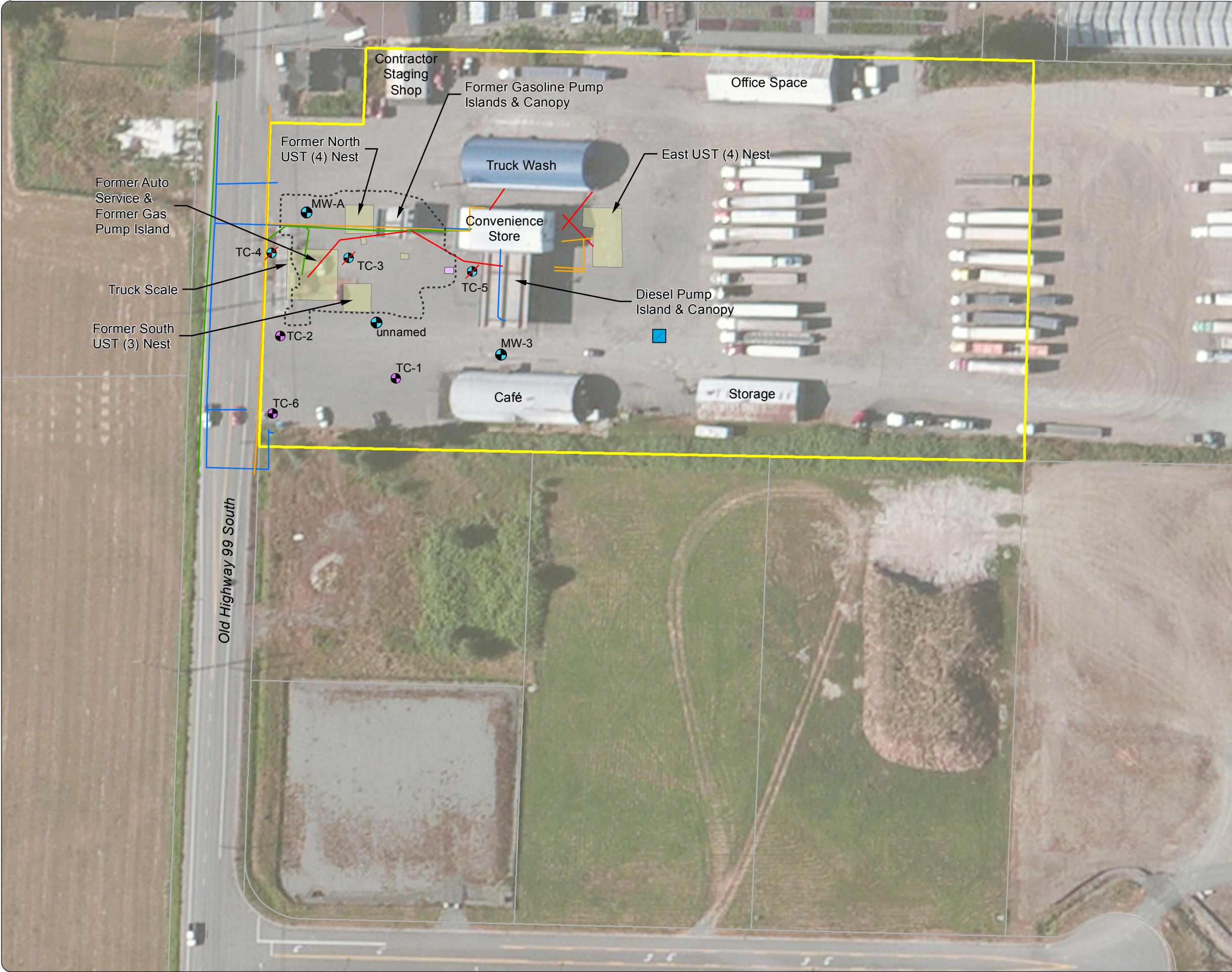
Figure 2-2 Pre-Remedial Action Site Features and Locations of MFA Investigation Former Truck City Site Mount Vernon, Washington
