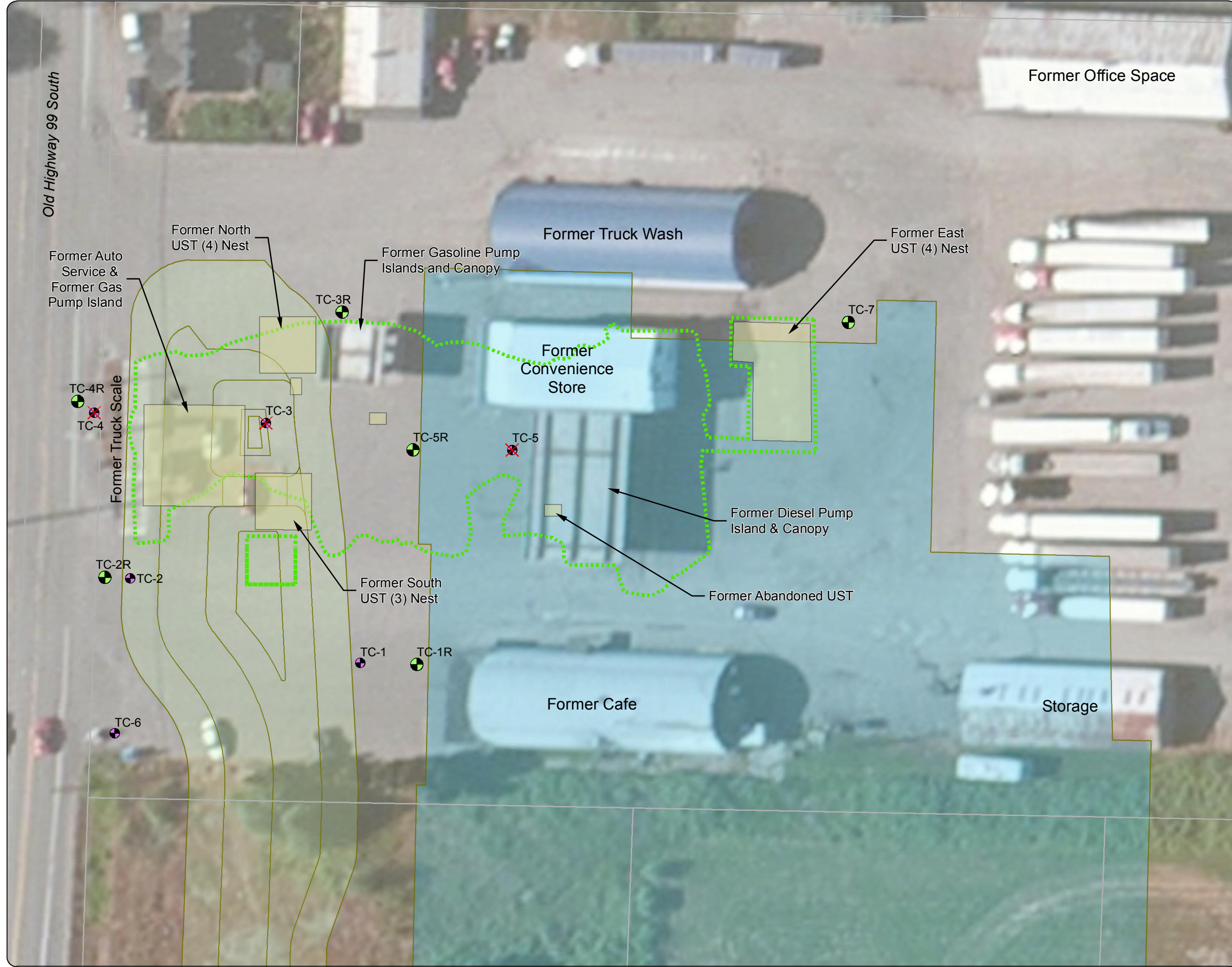
Figure 11-1 Proposed Replacement Monitoring Wells Locations
