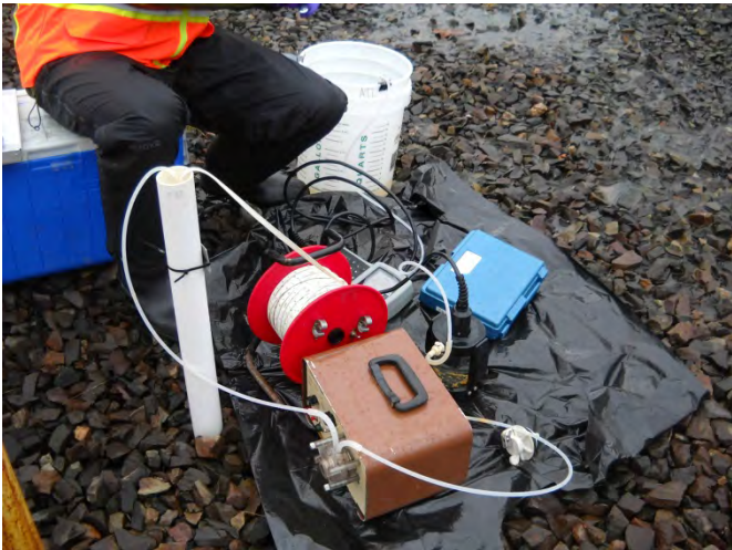
Photograph 11. Collecting groundwater samples during a monitoring event at the Seattle Terminal Properties.
