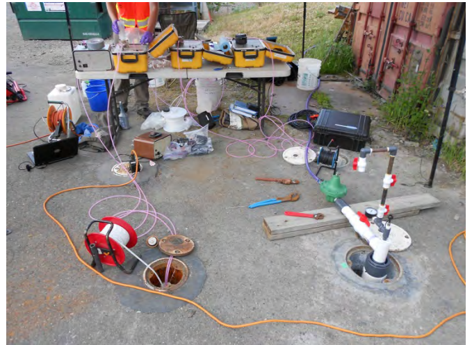
Photograph 12. Conducting a tracer study at the ASKO Hydraulic Property.
