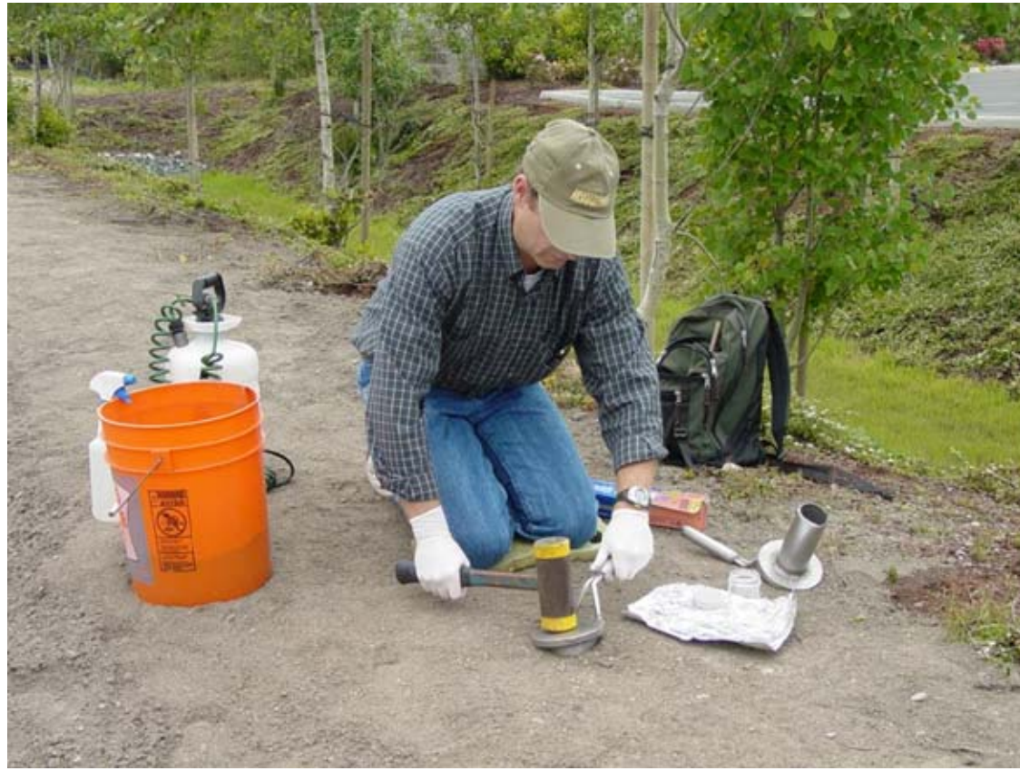
1. The sampler pounds a metal sampling tool into the ground.
