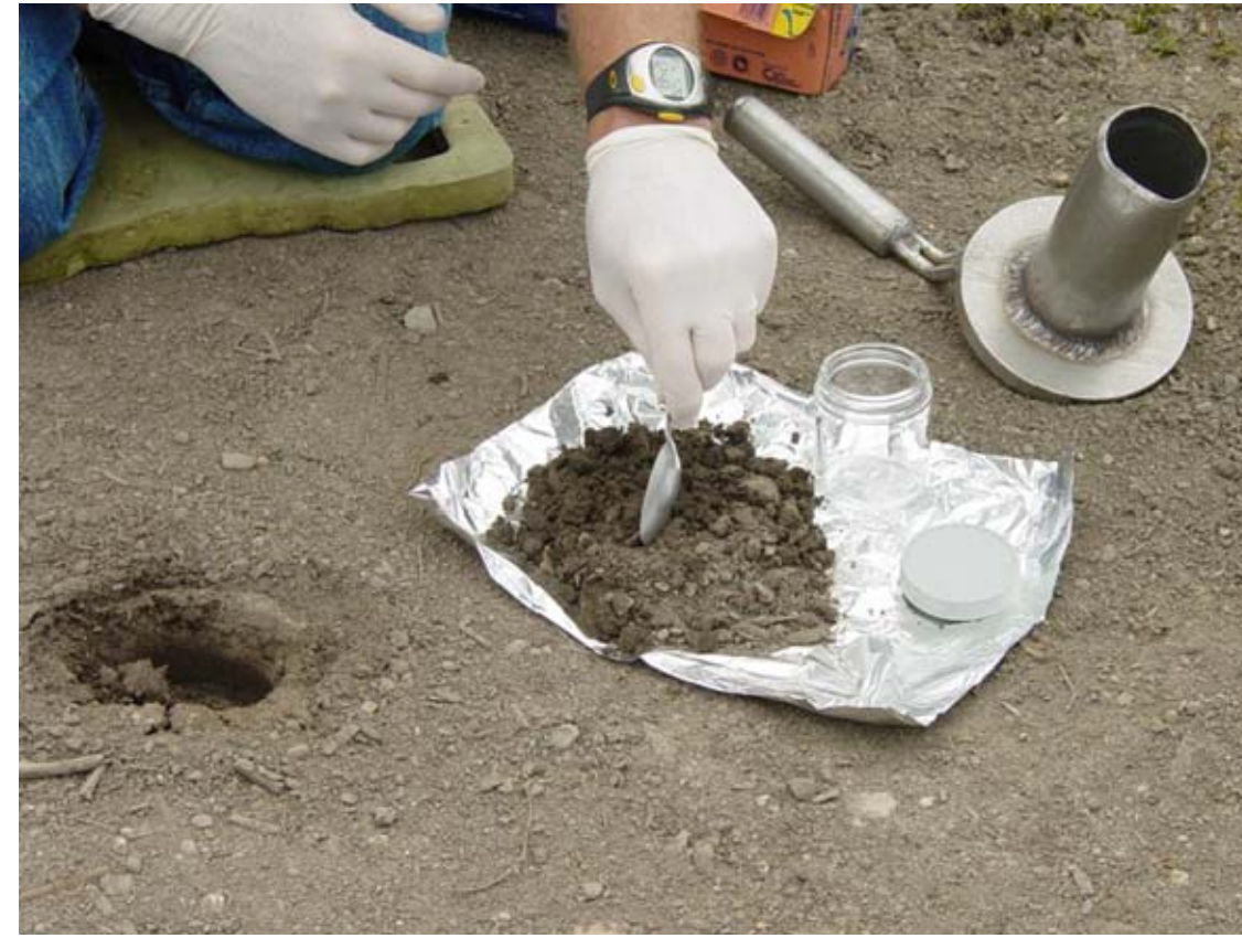
2. The tool pulls out a soil sample. Small rocks need to be removed.
