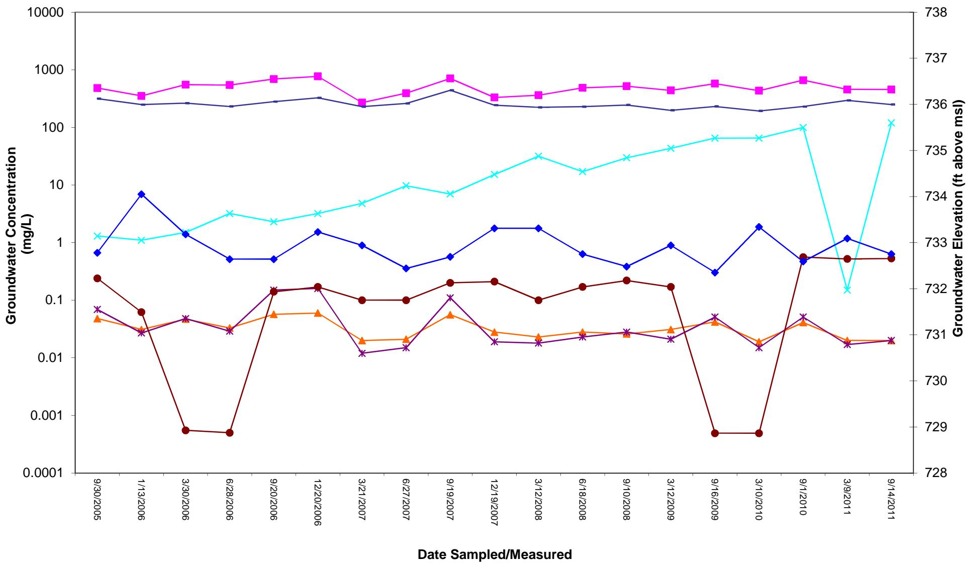
**MW-10 Groundwater Concentrations and Elevations vs. Time**
