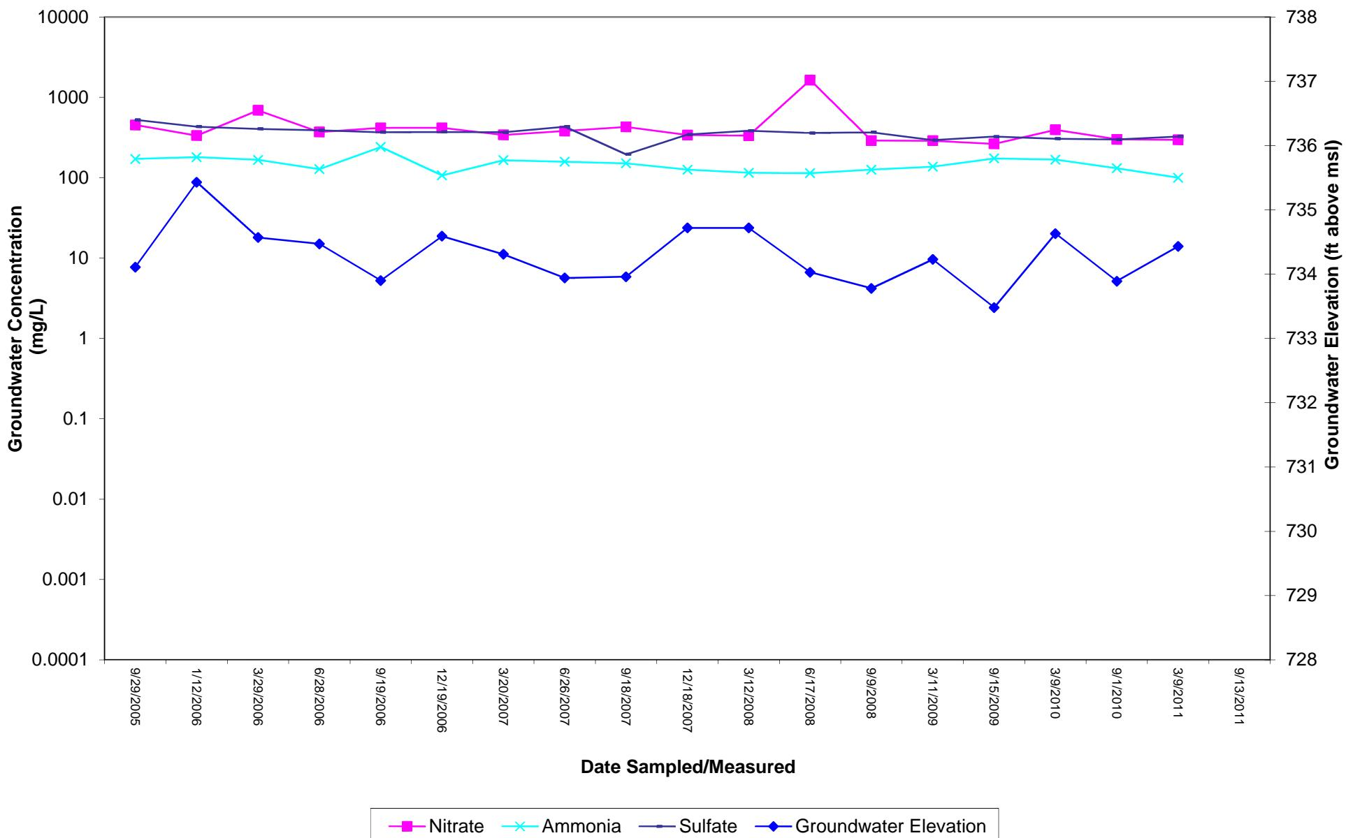
**MW-6 Groundwater Concentrations and Elevations vs. Time**
