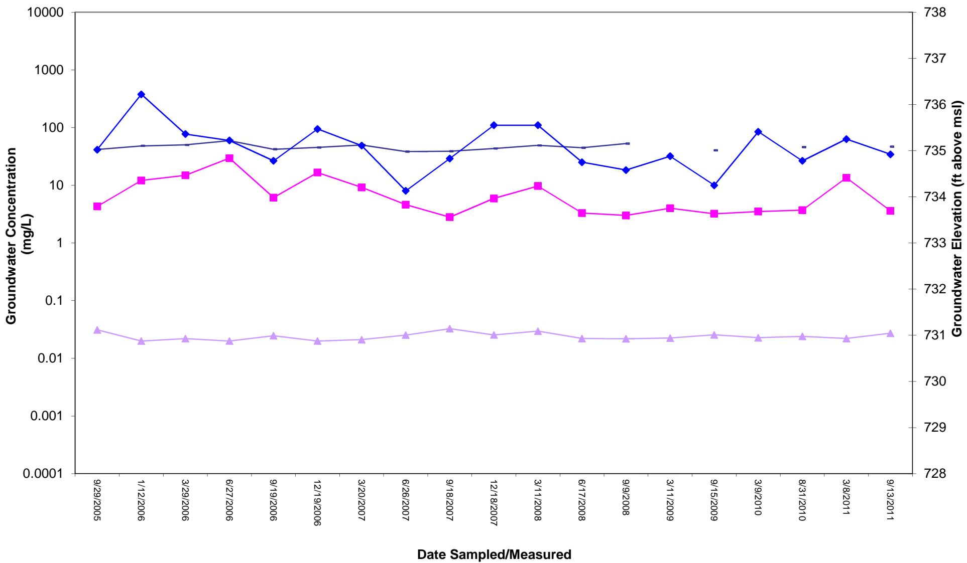
**MW-7 Groundwater Concentrations and Elevations vs. Time**
