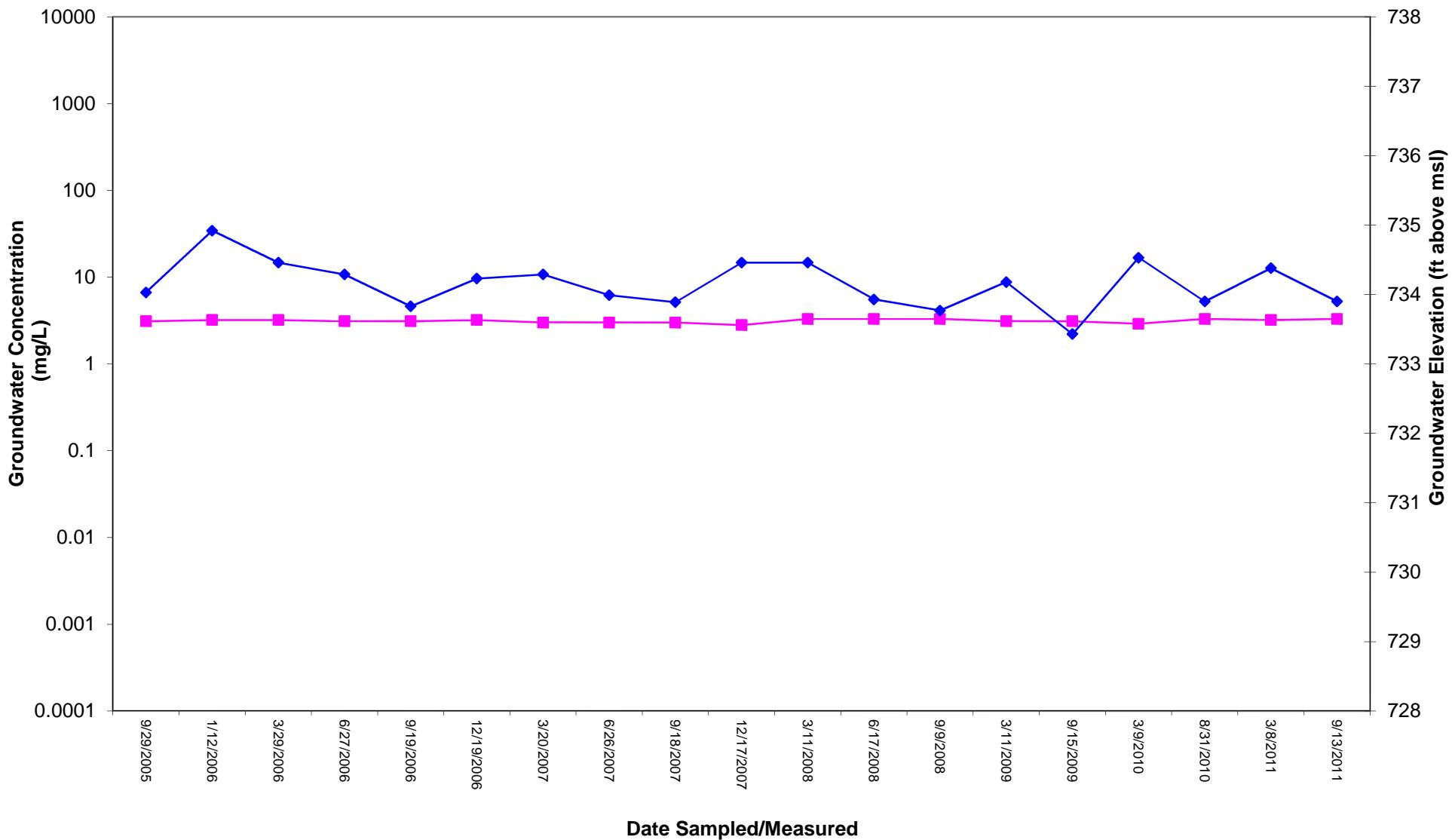
**MW-8 Groundwater Concentrations and Elevations vs. Time**
