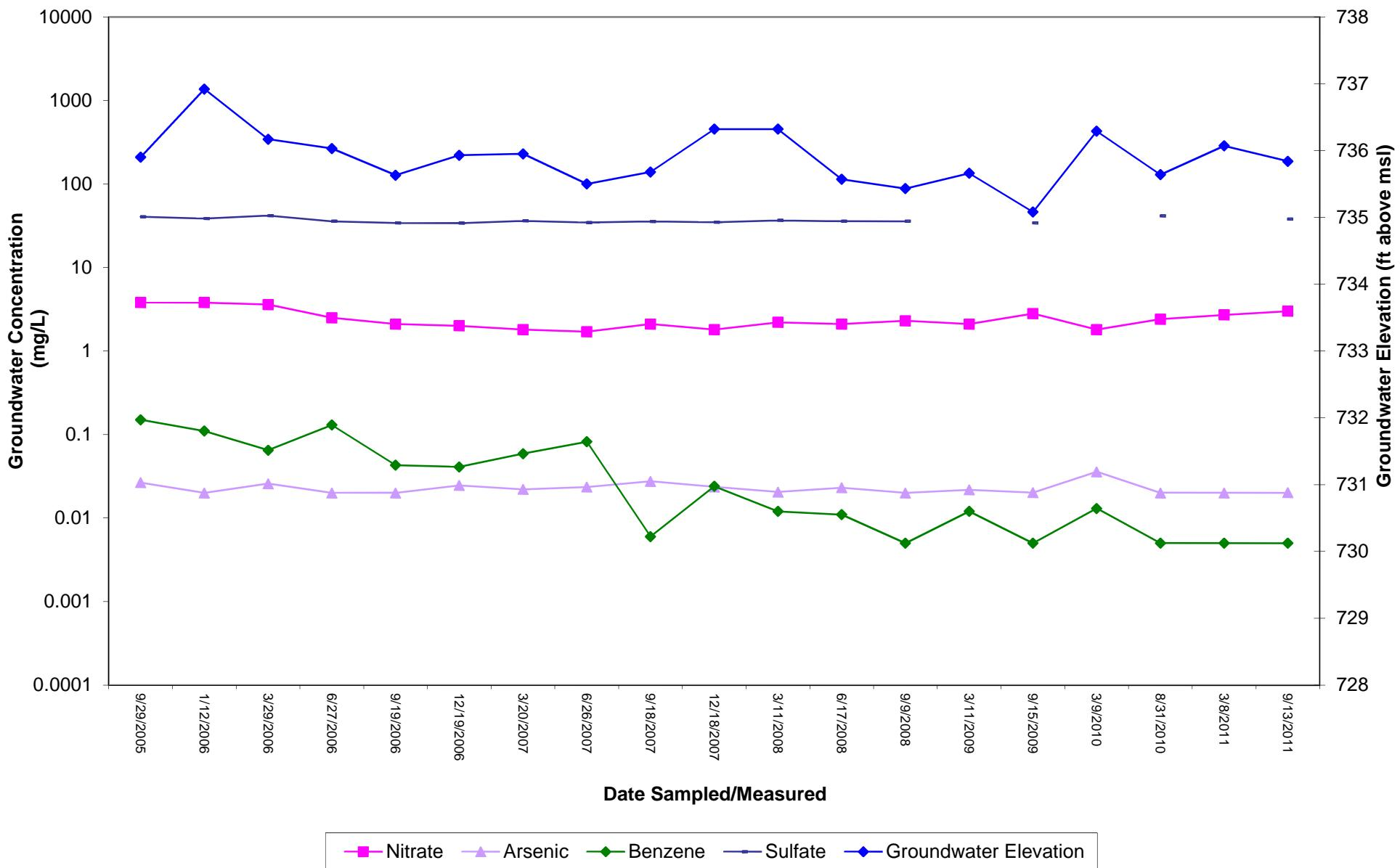
**MW-11 Groundwater Concentrations and Elevations vs. Time**
