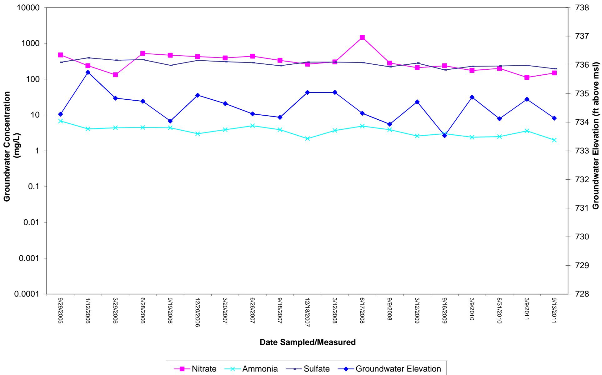
**MW-9 Groundwater Concentrations and Elevations vs. Time**
