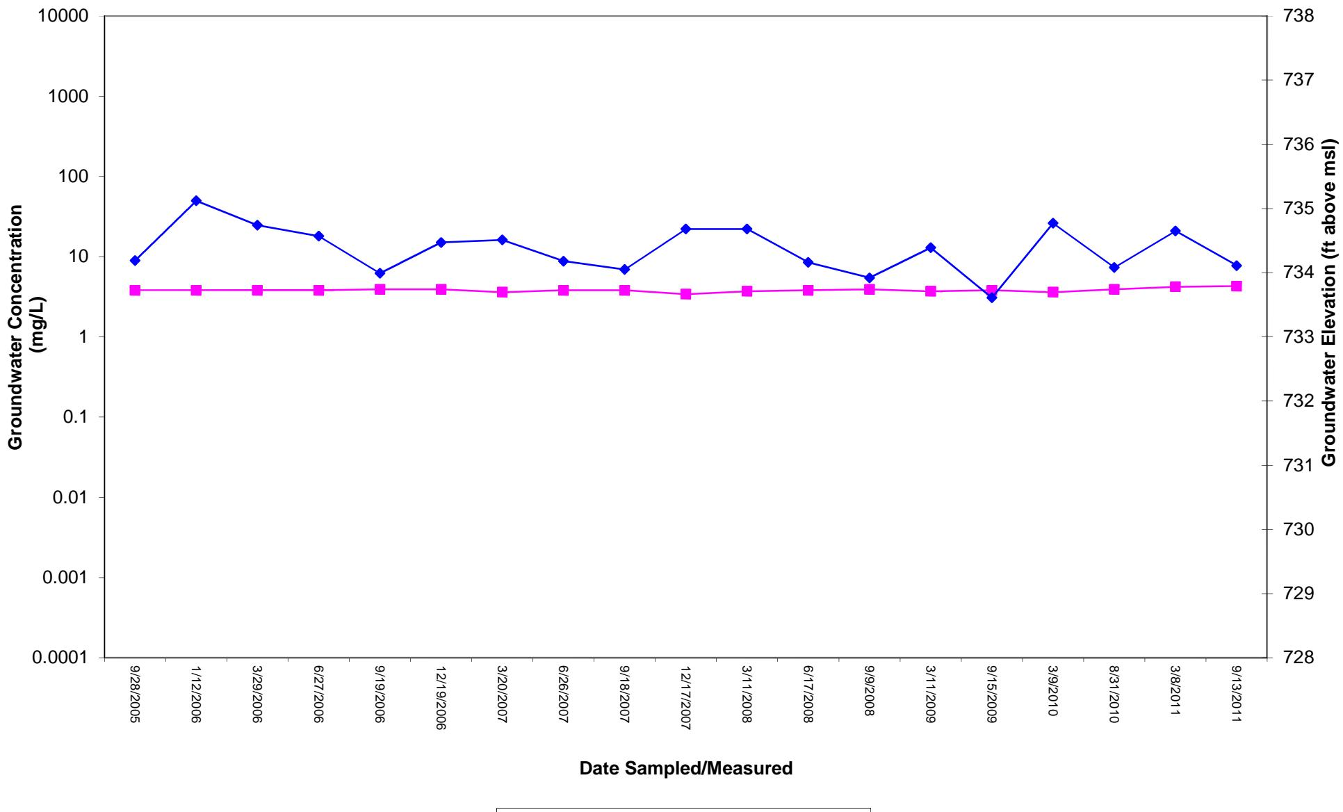
**MW-3 Groundwater Concentrations and Elevations vs. Time**
