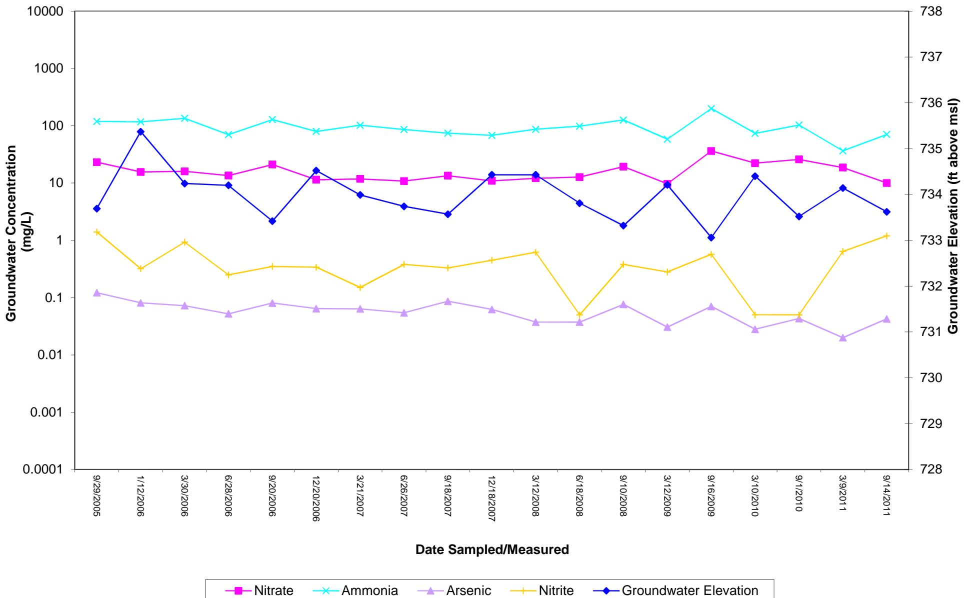
**MW-4 Groundwater Concentrations and Elevations vs. Time**
