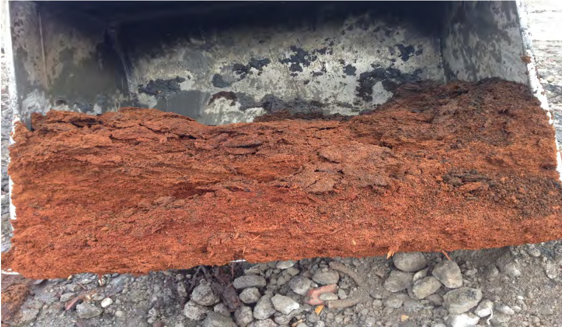
Photograph 11 – CN-B2 excavation: sawdust from deepest point of excavation
