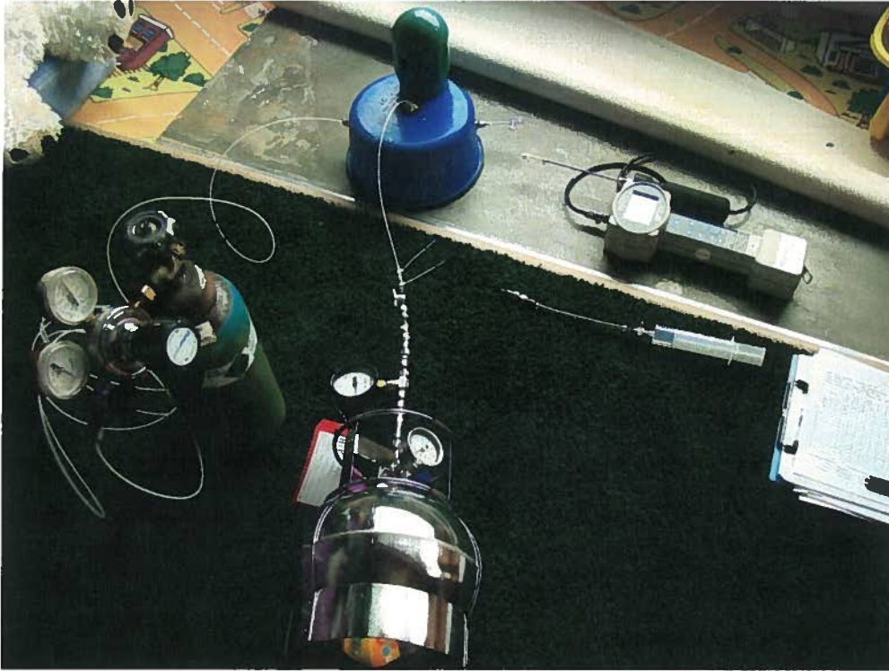
Photo #1: Purging and sampling equipment, including helium shroud for leak check, pictured during subslab soil gas sampling in the childcare center at location SS-1. (September 2011)
