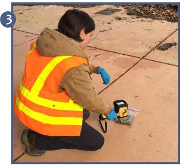
The samples are tested on site using the XRF tool to find out if arsenic is present above state cleanup levels.
