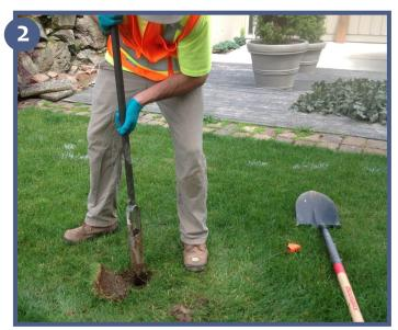
The auger takes a sample that is two inches in diameter and two feet deep. Crews may be in your yard for several hours to collect samples.
