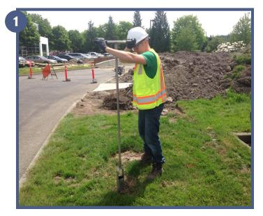
Ecology will enter your yard to collect multiple soil samples using a tool called an auger.
