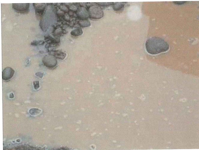
Photo 05 - Sheen observed on water during excavation
