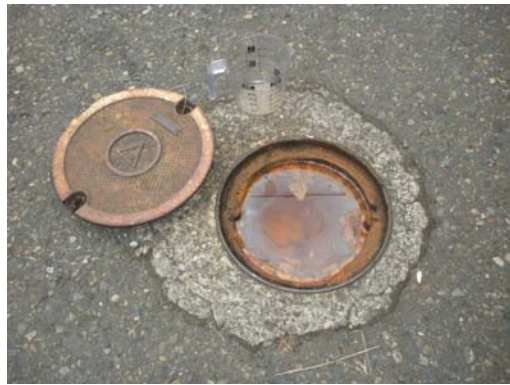
Photo 26 Top View Project Site MW - 4 Monument Full of Surface Water Water Was Removed Well Sealed w Cap
