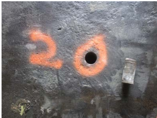
Photo 14 Top View Project Site First Addition Soil Sample 2 Core Removed Sub Slab View Typical
