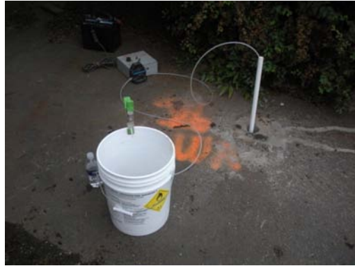
Photo 21 Facing North Project Site Water Sample WA-2 North of Drain Outlet 3/4 Inch Diameter Well Peristaltic Pump Waste Collection Pail Typical
