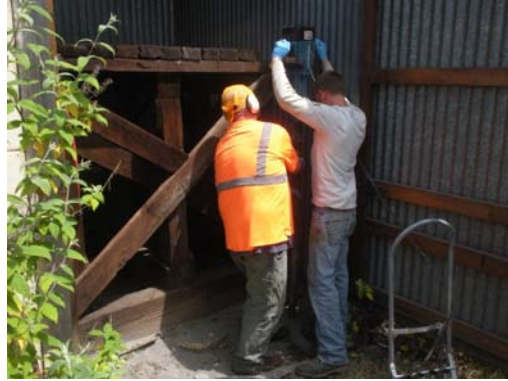
Photo 16 Facing East Project Site Second Addition Soil Sample 8 Hand Jack Hammer With Steel Soil Probe Beneath Acid Vessel Wooden Platform
