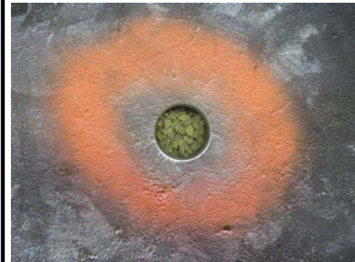
Photo 22 Top View Project Site After Soil Sample Bentonite Chip Seal Typical
