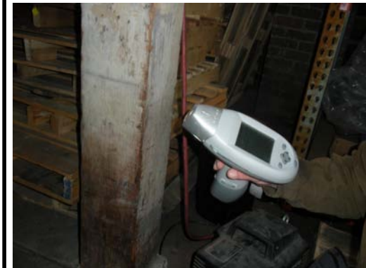
Photo 9 Facing West Project Site First Addition Hazardous Building Materials Survey XRF Testing Structure Timber
