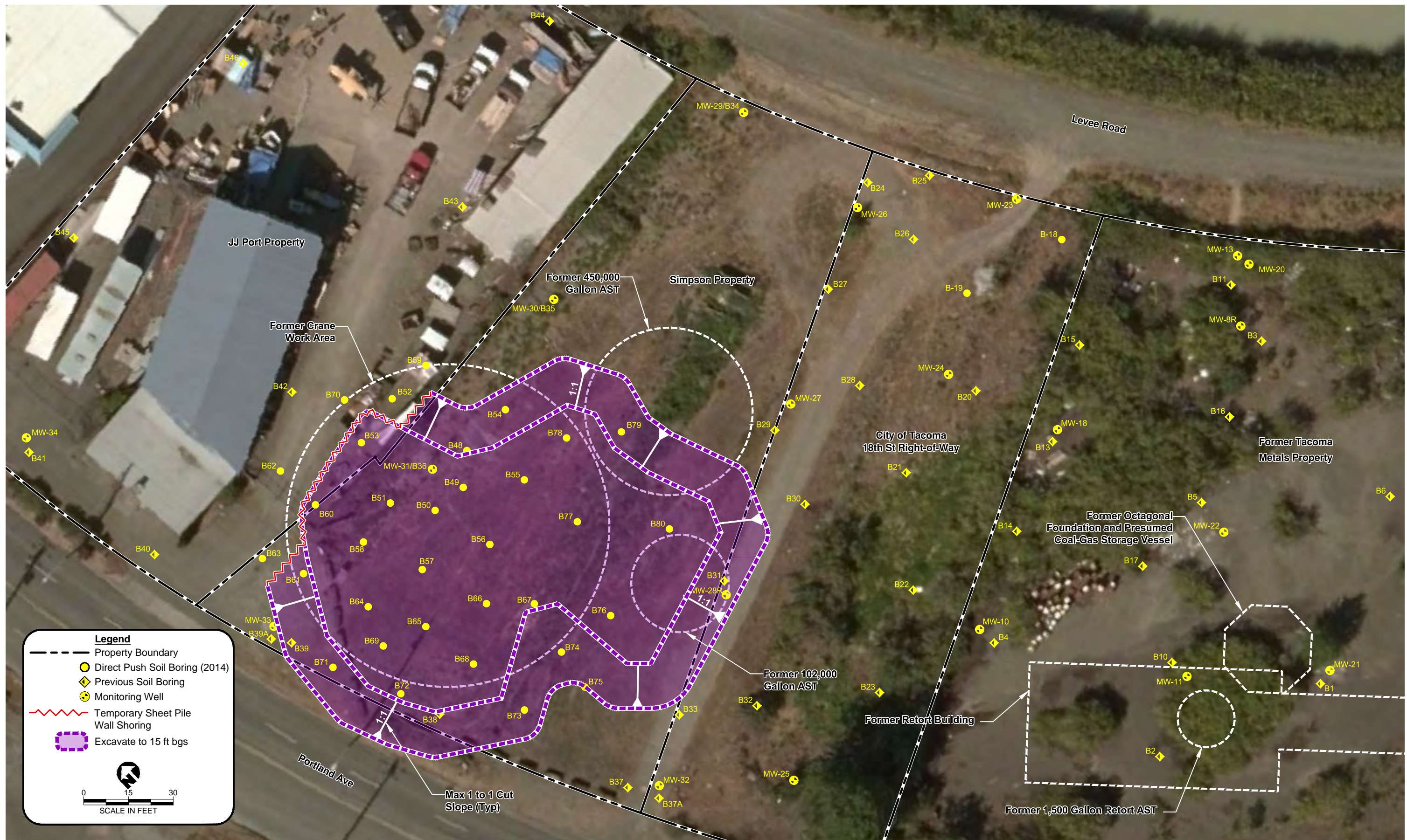
Figure 2-1 Alternative 1 Soil Excavation and Disposal
