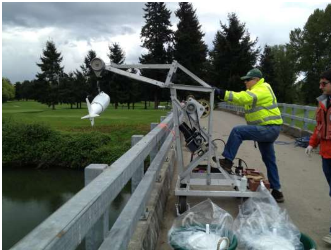
Figure 6. Photo of example USGS sampling equipment, including a crane, reel, and sampler for representative collection of depth- and width-integrated samples.
