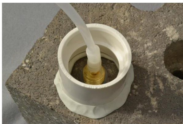
Figure 6. Water dam used for leak detection
