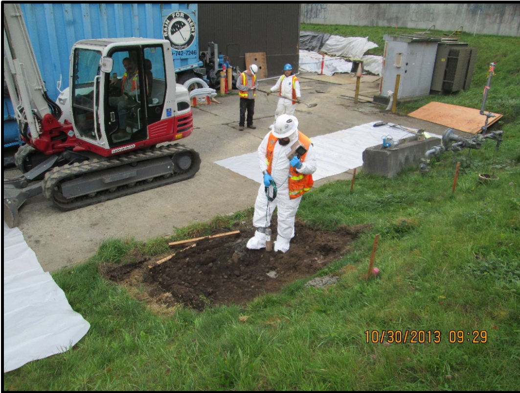
Photograph 1-7: Gamma walkover survey of hotspot excavation west of Building 27.
