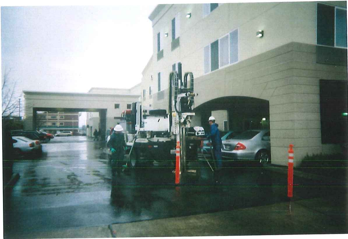
Direct push sampling system at borehole sampling location S-6
