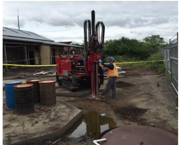
Crew installing a temporary borehole for soil and groundwater-grab sampling using a push probe. Located in the former tank farm. Photo by David Coles.
