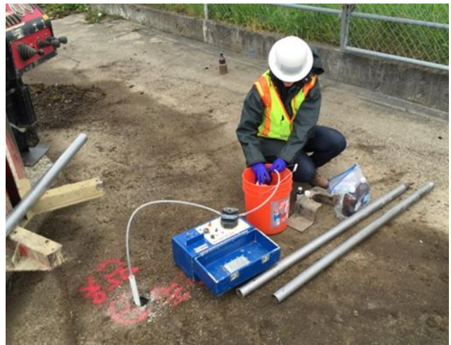
Geologist Jill Betts, LG, sampling groundwater from a temporary boring with a peristaltic pump. Photo by David Coles.
