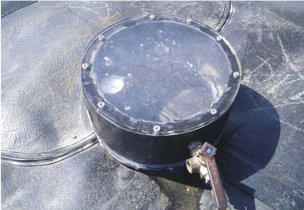
30166 June, 2004 – Vacuum chamber box for testing extrusion fillet welds. The box, with a transparent lid, applies a vacuum of approximately 3 psi to weld. Soap solution placed over weld prior to application of vacuum will bubble if weld is not constructed correctly.
