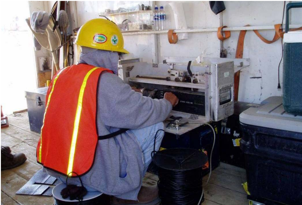
50066 May, 2004 – Field testing of test specimen weld using a field tensiometer. Specimen is tested in peel and shear modes until failure and result is compared with manufacturer's values for conformance.
