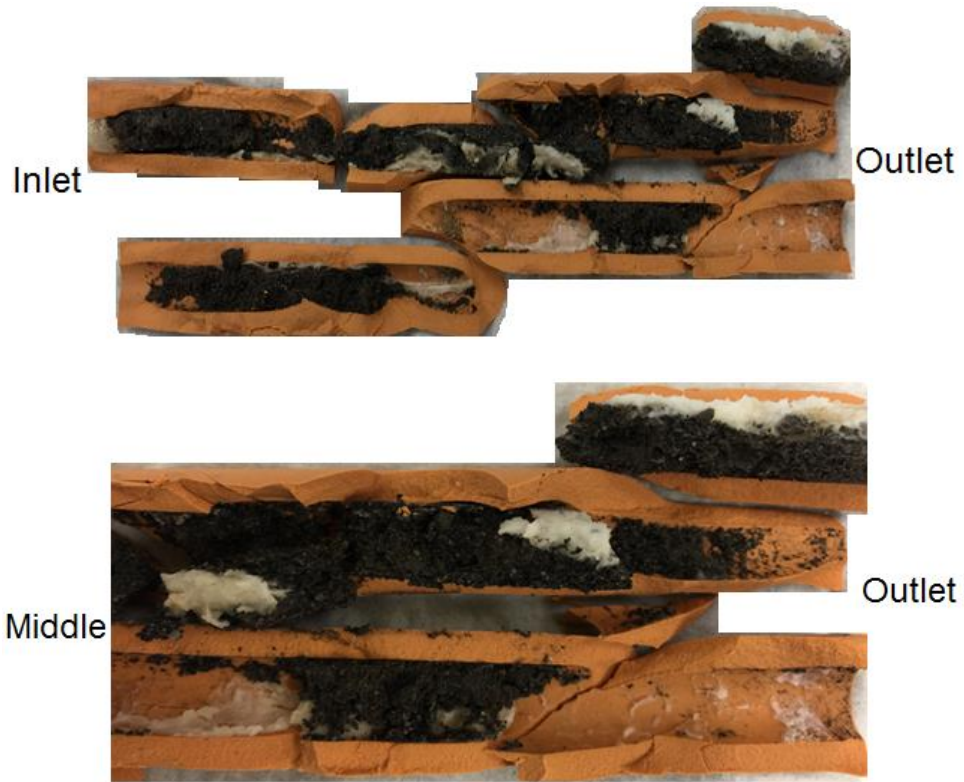
Figure 76 View of the cross-section of a split soil column after injection of 1 M \text{NaHCO}_3 .
