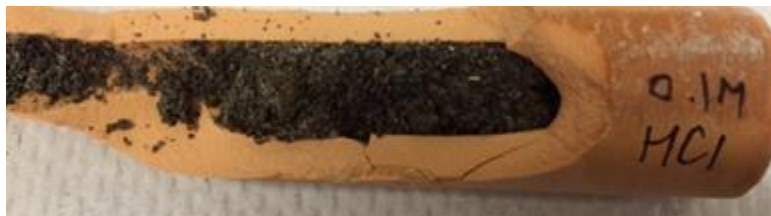
Figure 73 General view of the contents of soil column after injection of 0.1 M HCl.
