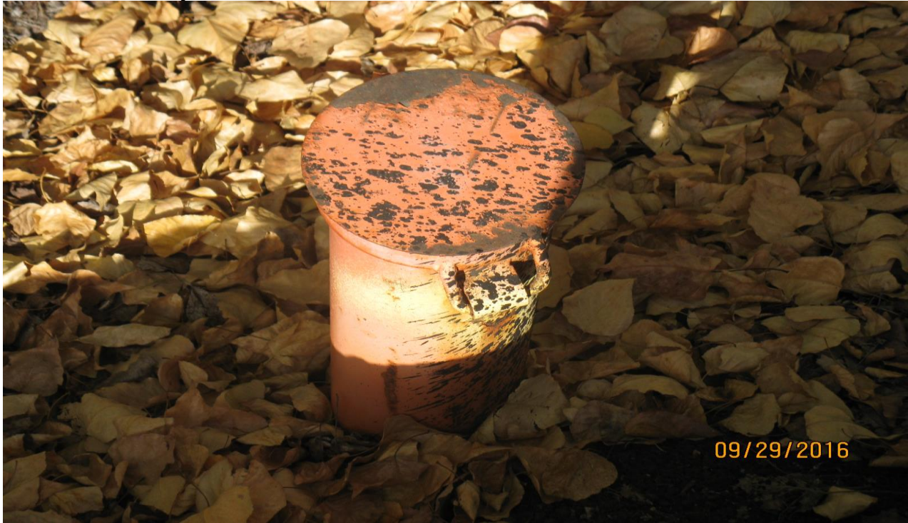
Photo 7: Downgradient Groundwater Monitoring Well, MW-2 at the Western Property Boundary of the Site
