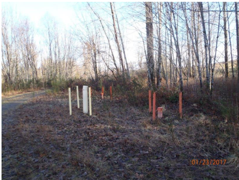
Photo 8: Groundwater monitoring wells and gas monitoring probe
