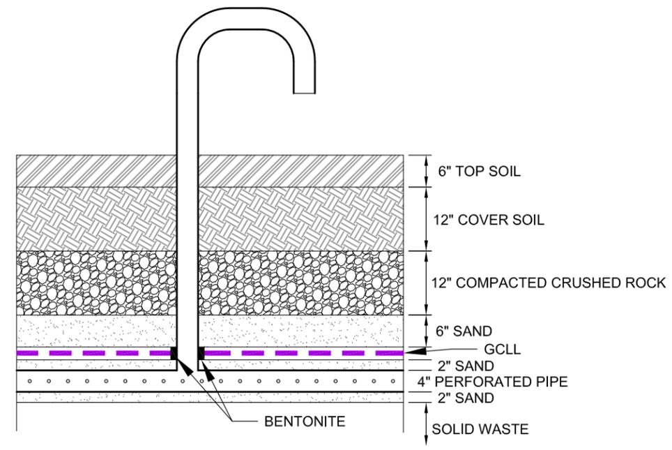
2 PASSIVE LANDFILL GAS VENT DETAIL
