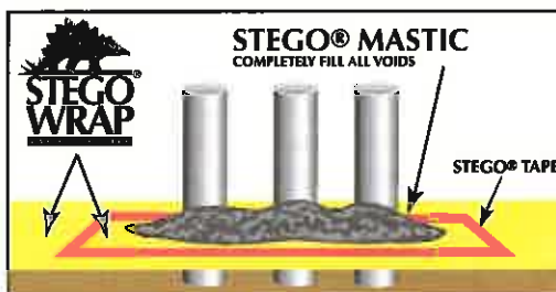
FIGURE 5: MULTIPLE PIPE PENETRATION SEALING
