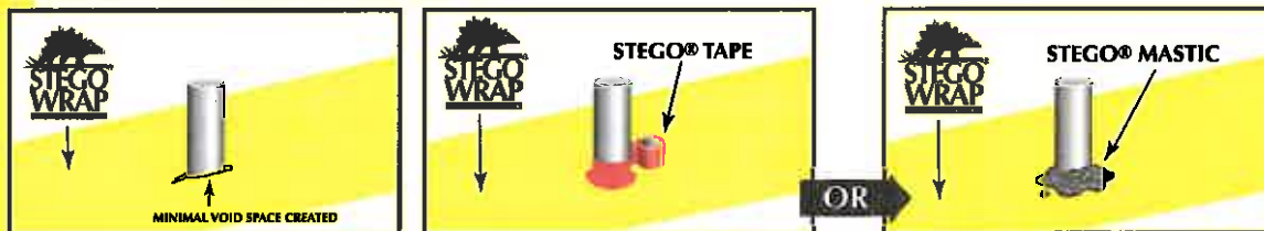
FIGURE 4a: PIPE PENETRATION SEALING
