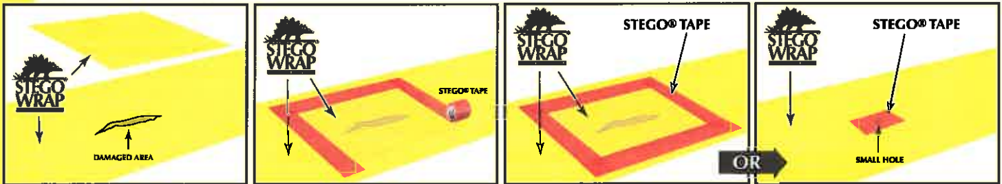
FIGURE 3: SEALING DAMAGED AREAS
