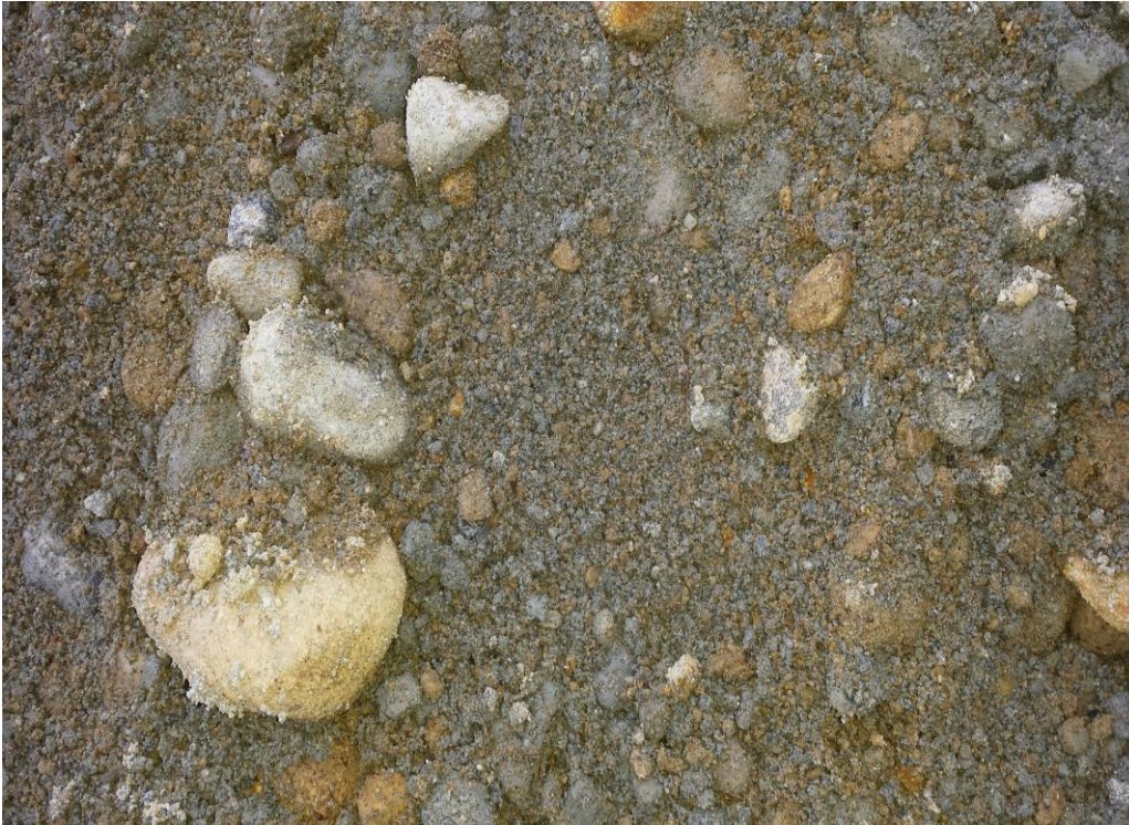
2. Soils initially observed were fill materials. Beneath the fill were brown and gray, damp, medium dense sand with gravel and minor silt (USCS SP to SM).
