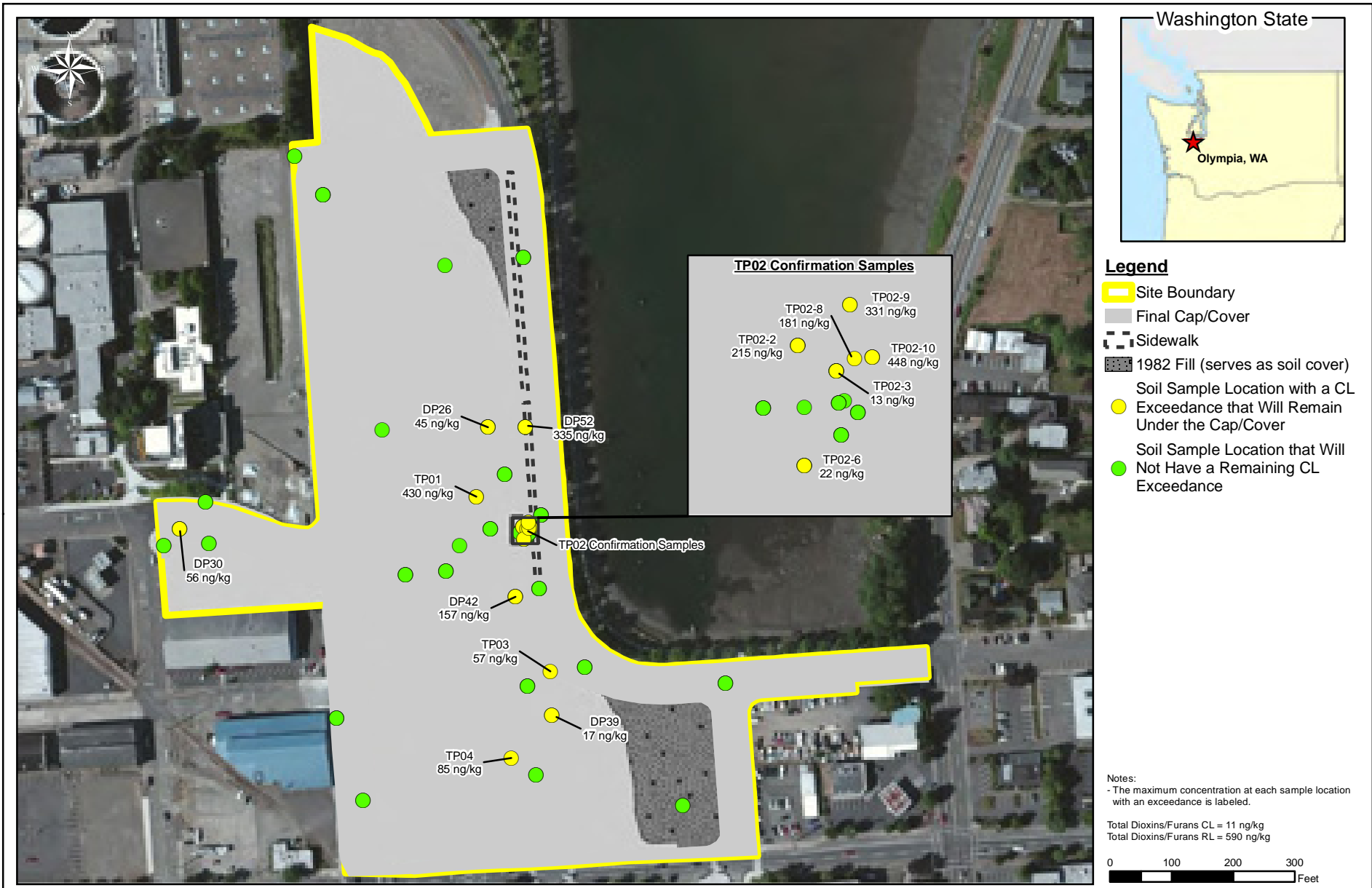
Total Dioxins/Furans Cleanup Level Exceedances That Will Remain Cleanup Action Plan East Bay Redevelopment Site
