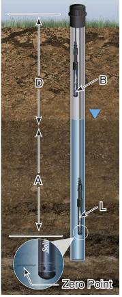
A = L - B Figure 1-1 Levelogger Measurement Fundamentals
