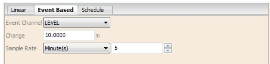
Figure 5-10 Event Based Sampling Setup
