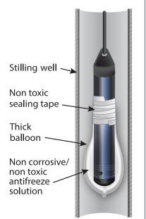
Figure 10-16 Installation in Freezing Liquid
