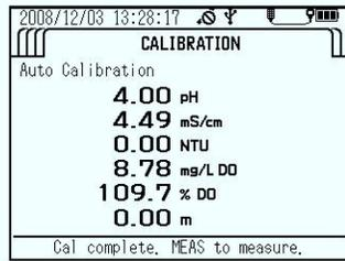
6. Press the **MEAS** button to display measured parameter values. Record, at a minimum, values for pH, turbidity, conductivity, and dissolved oxygen (values for temperature, salinity, and oxygen reduction potential (ORP) may also be recorded to evaluate meter). Expected parameter value ranges are as follows:
