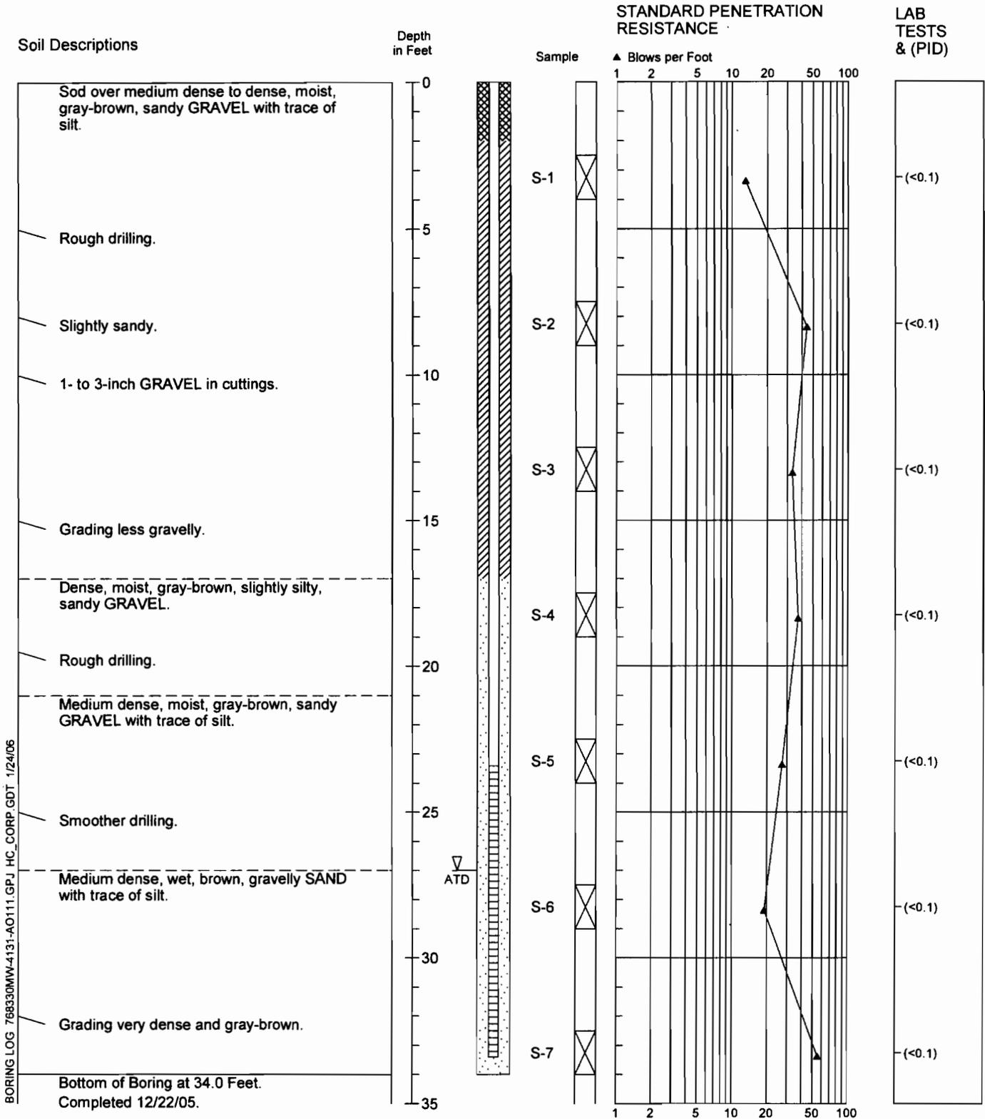
BORING LOG 768330MW-4131-AO111.GPJ\_HC\_CORP\_GDT\_1/24/06
