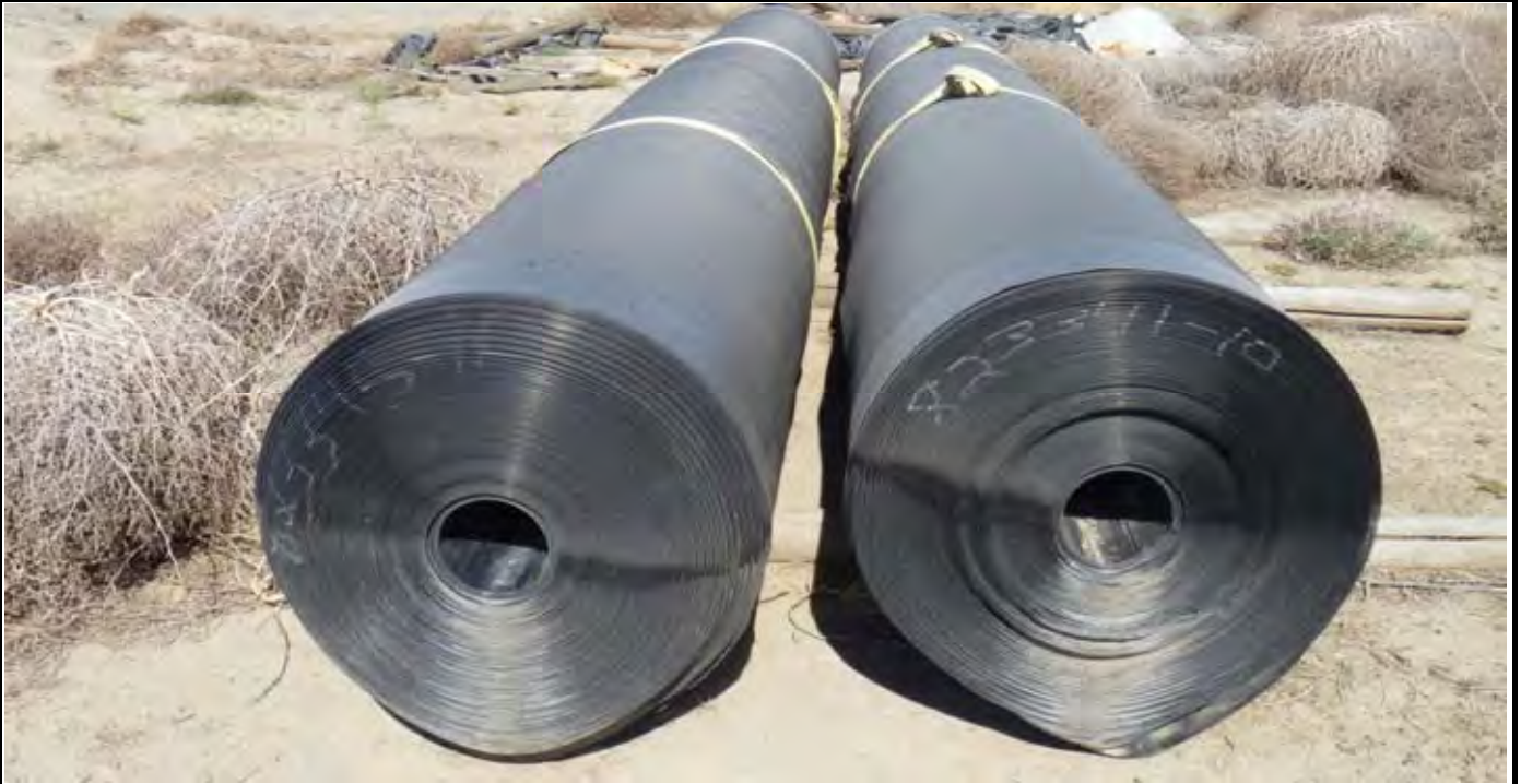
Photo 3: View of the two geomembrane rolls from original work that are accepted by geosynthetic vendor. See field notes for specs/roll number. Rolls located up on roadway near original g-layer stockpile area. View looking west.
