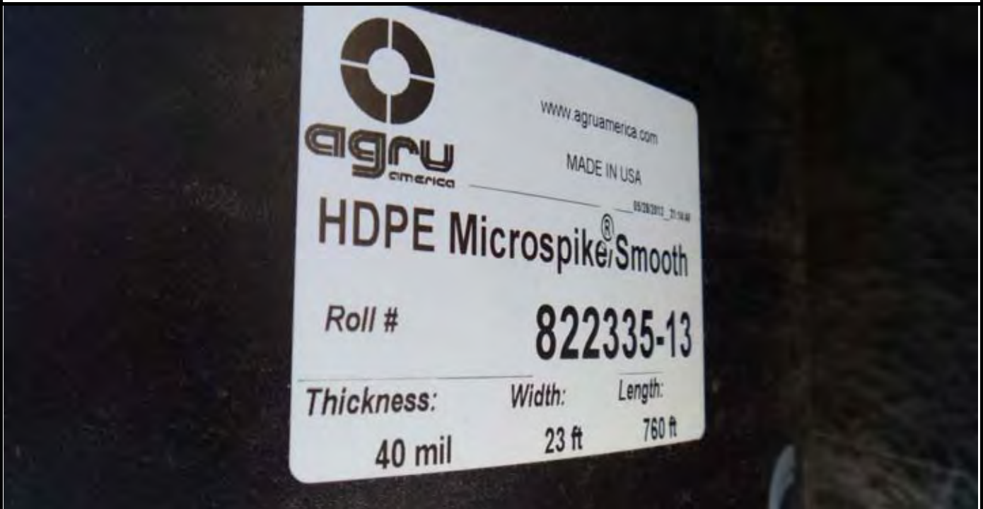
Photo 6: View of label on second roll of 40-mil HDPE Microspike / smooth geomembrane. Roll # = 822335-13 Thickness = 40-mil, Width = 23-ft, Length = 760-ft for a total area of roll = 17,480-sf Microspike side is considered "textured".
