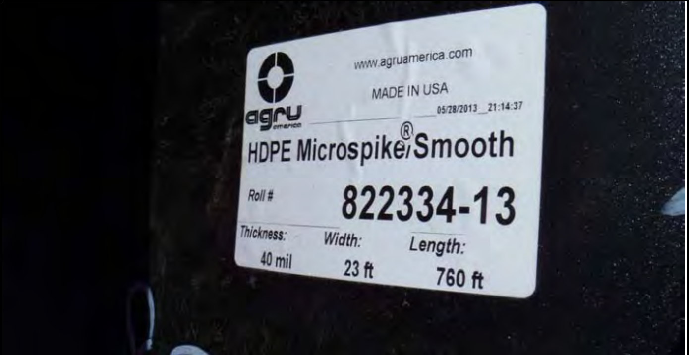
Photo 5: View of label on first roll of 40-mil HDPE Microspike / smooth geomembrane. Roll # = 822334-13 Thickness = 40-mil, Width = 23-ft, Length = 760-ft for a total area of roll = 17,480-sf Microspike side is considered "textured".
