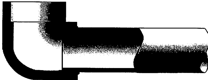
Figure 4 Standard Socket Fusion Joint
