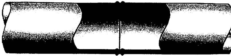
Figure 1 Standard Butt Fusion Joint
