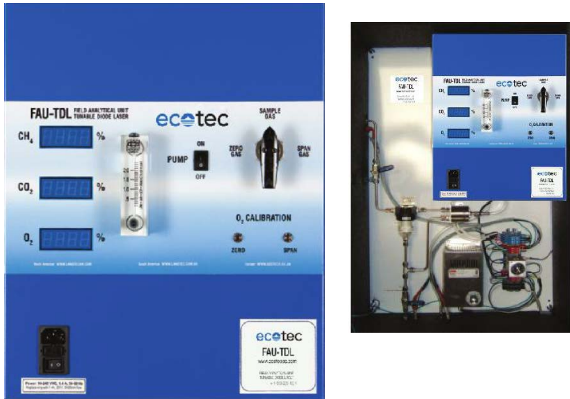
LFG Analyzer Display Screen and View of Internal Control Panel
