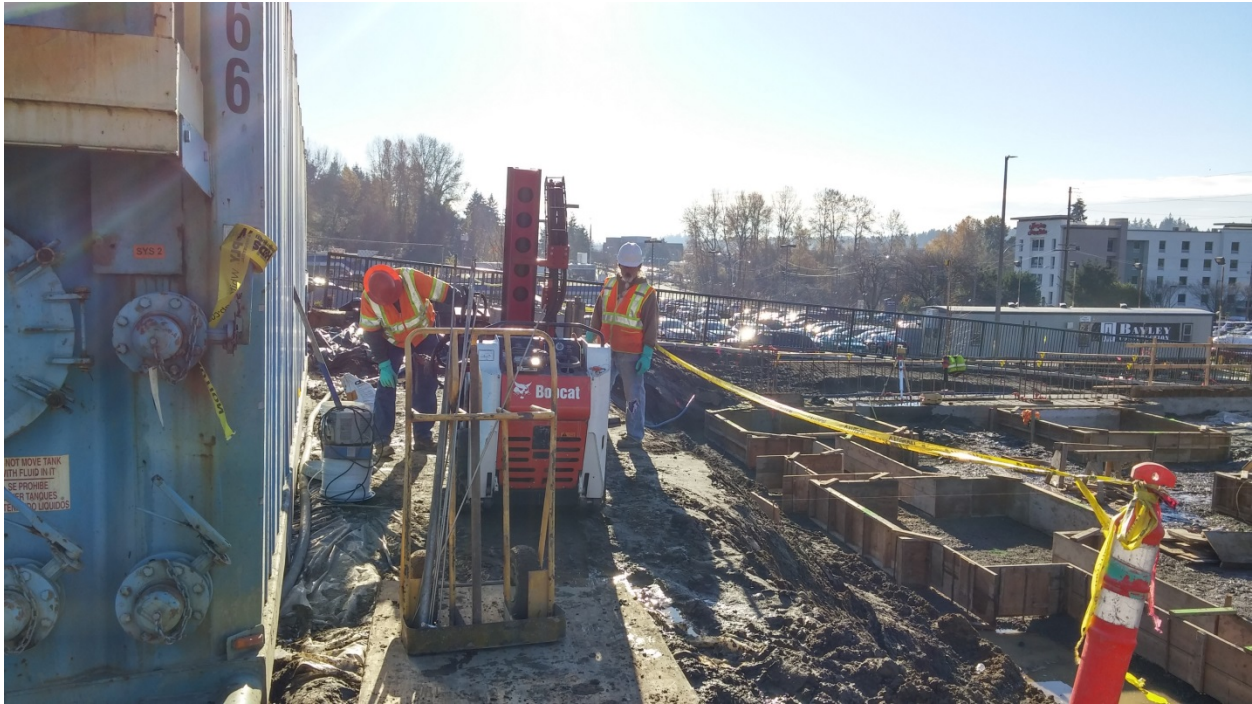
Photo 15: November 30, 2015. View of the limited-access direct-push sampling rig that was used to collect groundwater samples from five locations within the footprint of the main remedial excavation. Diesel- and oil-range TPH were detected below MTCA Method A cleanup levels.
