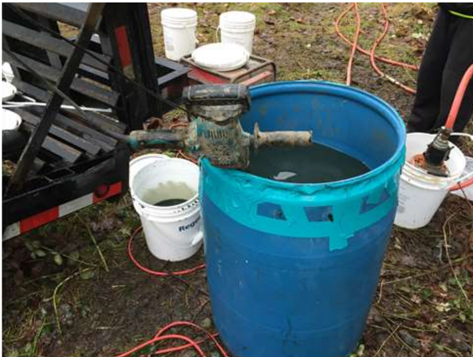
Photo 4 Looking northeast, plastic mixing barrel with RegenOx Part B mixture, electric stir tool set into barrel, electric submersible pump in white bucket to right.
