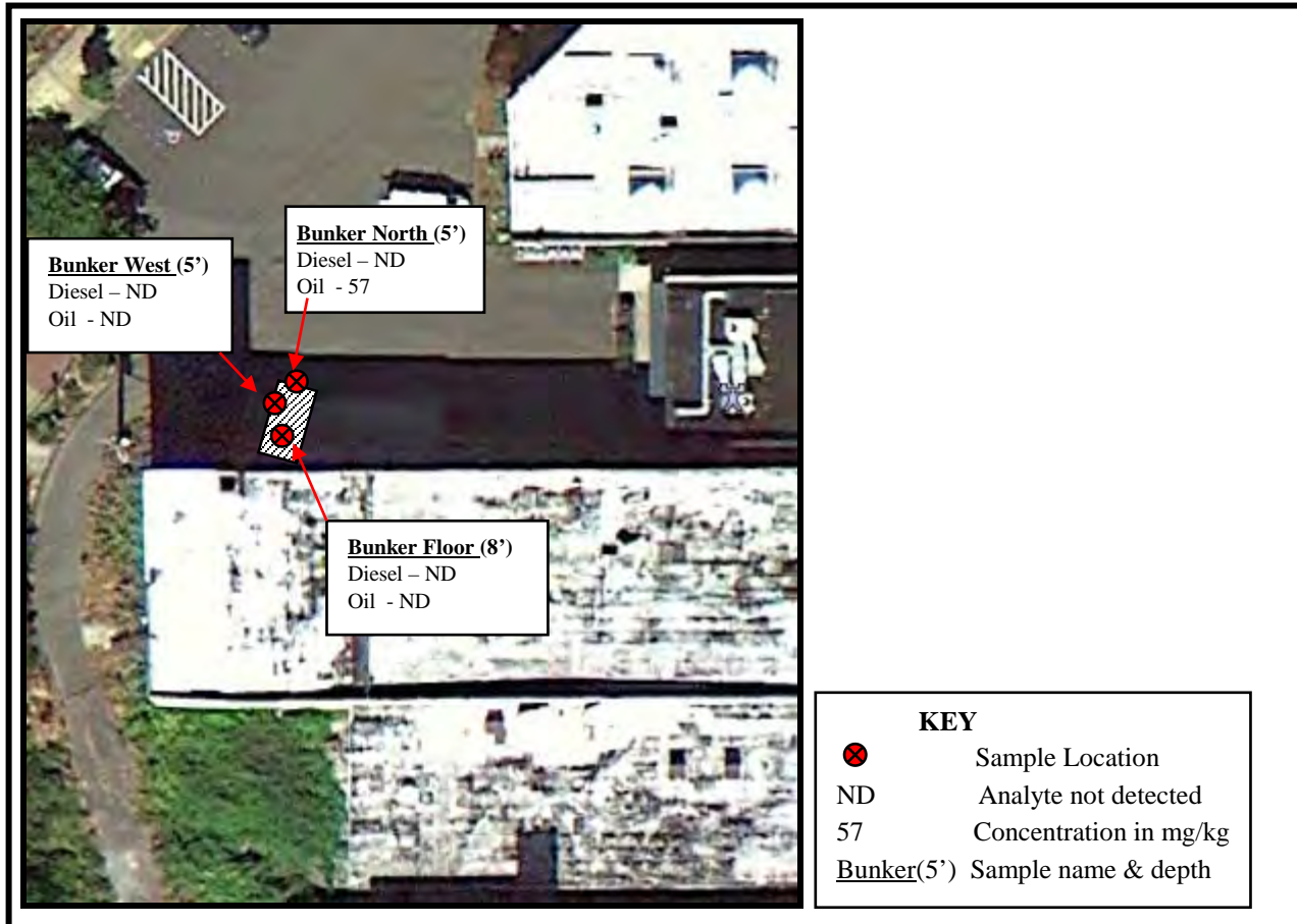
Figure 5. Sample results from heating oil UST removal
