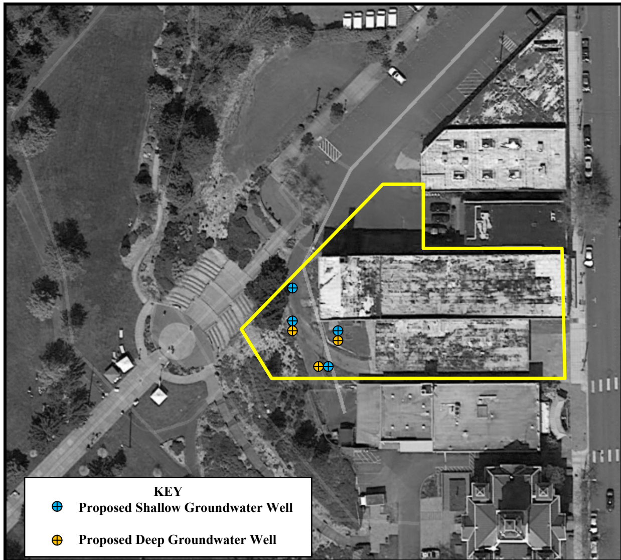
Location of proposed groundwater monitoring wells on the Cascade Laundry site
