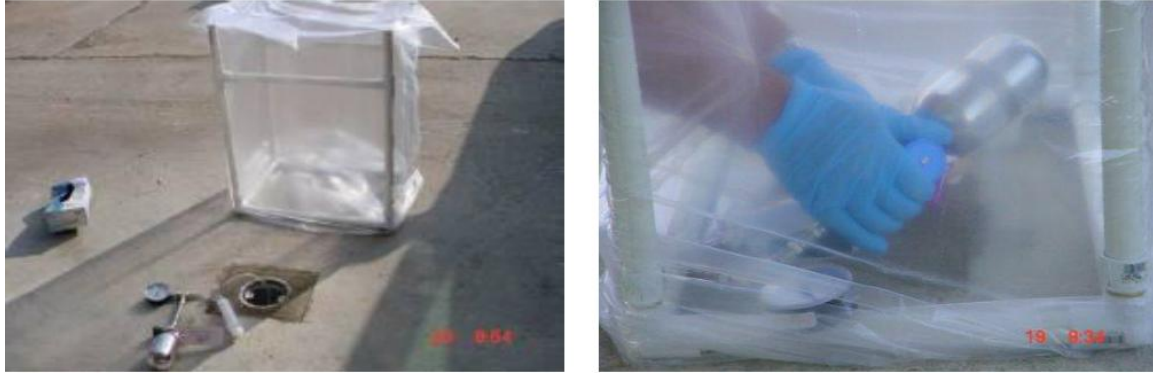
Figure 7. Helium shroud used for leak-testing soil vapor sampling train.
