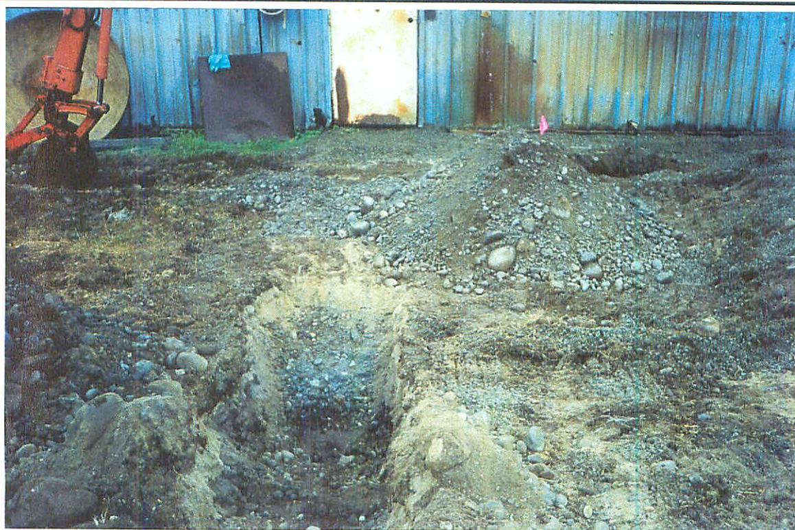
Photo #4: View of blue-gray and black-grey contaminated soil layers in Trench #2 (foreground), facing west. Trench #1 is on the right side of the photograph and Trench #3 is on the left. Photo taken on 10/03/02.
