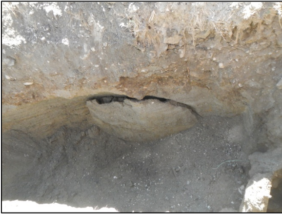
Test Pit TP-7: View of sidewall of completed test pit. Upper portion of photo is fill. Lower portion is beach deposits.
