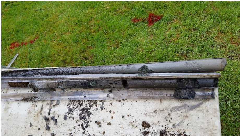
Soil cores and staining present in the samples from B8.
