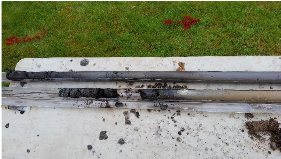
Soil cores and soil staining present in samples from B7.
