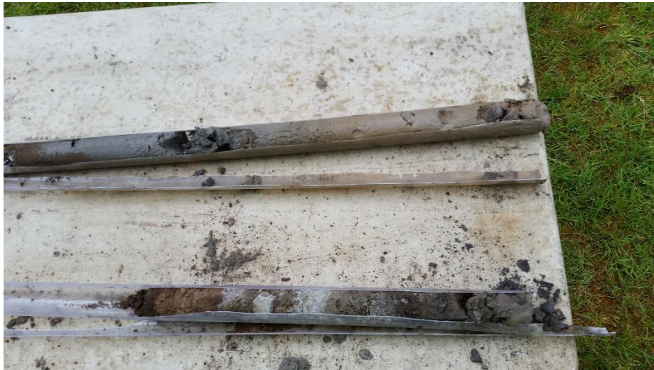
Soil cores from Borehole B5.
