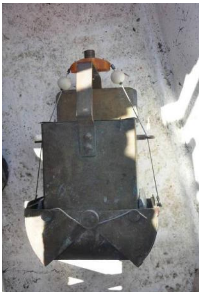
Photo 3: Ekman Dredge used to collect samples from bottom of river in pools.
