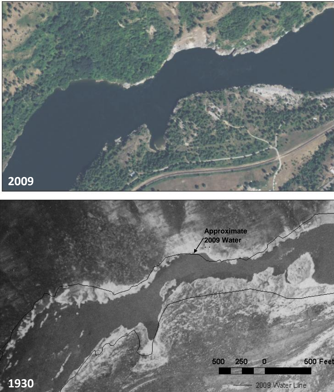
Figure 8. Aerial photos of the Little Dalles before and after channel modifications
