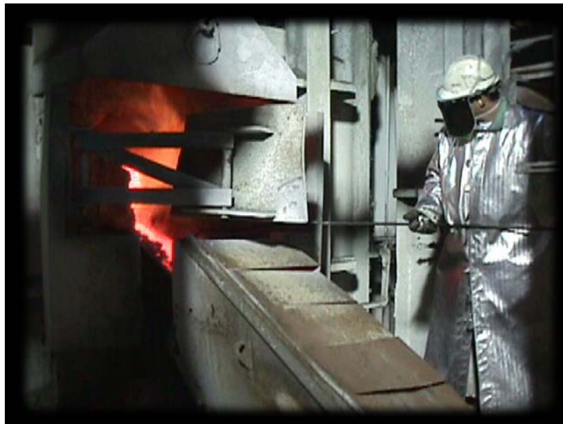
Figure 10. Tapping a reverberatory furnace (Queneau, CSM class slide)
