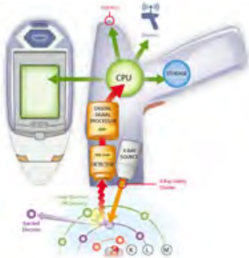
Figure 2. --- This shows the overall XRF process. High energy X-rays are directed at the sample and an atom ejects one of its low energy inner-shell electrons. That vacancy is immediately filled by a high-energy electron from an outer shell. The energy difference between the two is released in the form of lower-energy X-ray radiation, which enters the detector. The resultant electrical signal is sent through the digital signal processor and on to the CPU. Results are shown on the display and stored for downloading.
