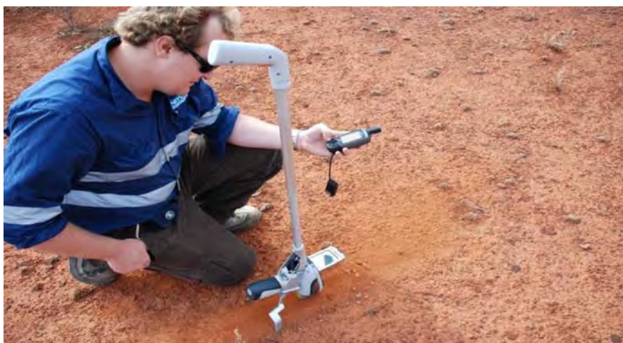
Figure 3. In-situ testing of soil by placing XRF directly onto the ground. This type of testing is generally screening level data quality.
