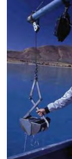
Ponar dredge using a winch
