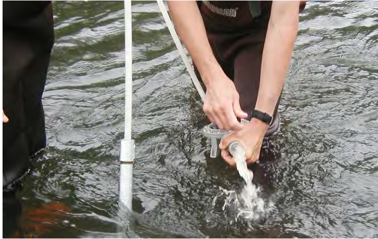
Figure 3 – Bilge pump development of a steel piezometer
