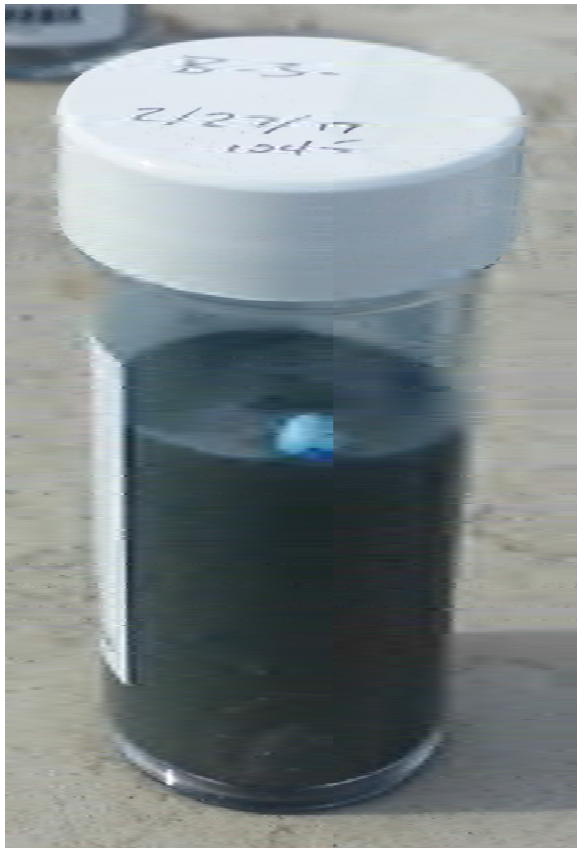
B-3 near water table: note blue dye on indicator bead and blue LNAPL blebs in suspension
