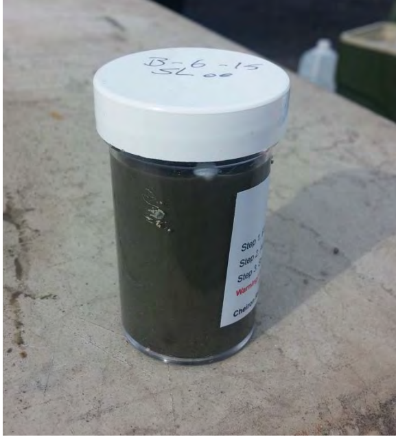
B-6 at 15ft bgs: Note lack of dye coloration on indicator bead indicating that petroleum concentrations at 15 ft bgs, below silt layer at 13-14 ft bgs, are not sufficient to be detected in the field test kit.
