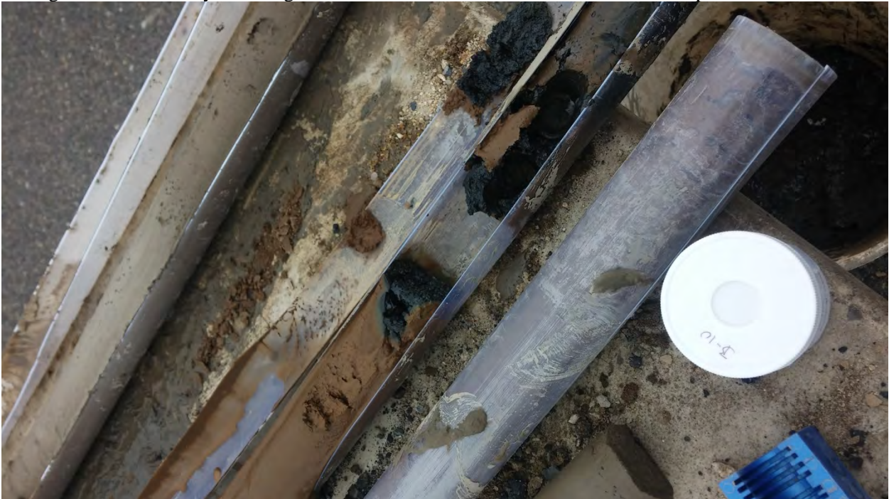
Boring B-10. Heavily petroleum-stained interval is at base of recovered core from 5-10 foot core interval, and the top of the impacted interval is likely located near the water table (approximately 8 ft bgs).
