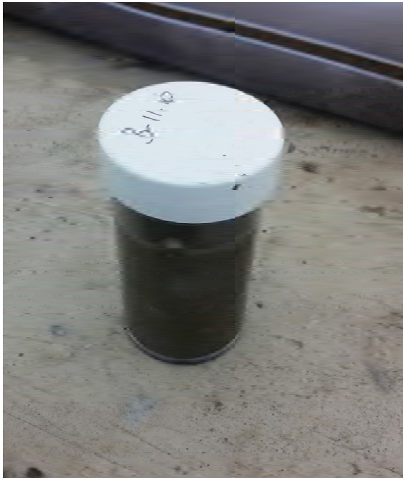
Boring B-11. Note lack of staining on indicator bead.
