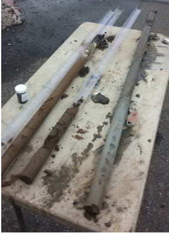
Boring B-4: note light gray silty interval in far right core (10-15 ft bgs), and poor recovery in middle core (5 to 10 ft bgs), which would span the water table interval. The top of each core interval is at the far end of the table. The light gray silt interval did not exhibit obvious petroleum odor, and the coloration appears to be natural, and consistent in all locations/borings it is observed in at the site.
