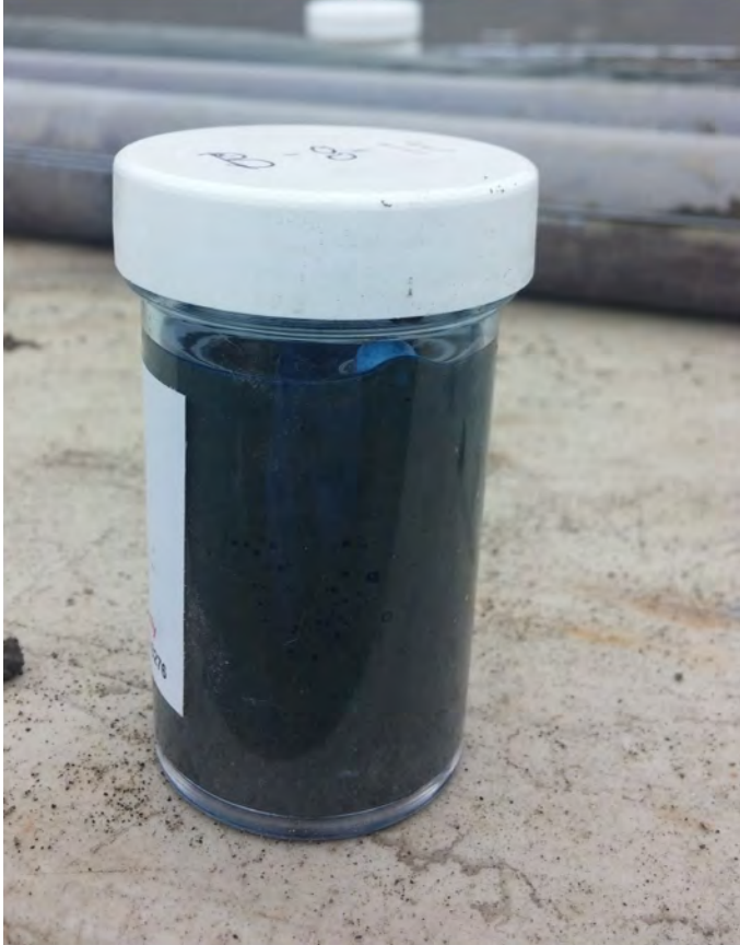
Boring B-8. Note blue dye staining on indicator bead and blue LNAPL blebs in suspension.
