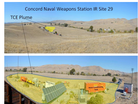
Figure 1: TCE plume at IR Site 29 at Concord Naval Weapons Station
