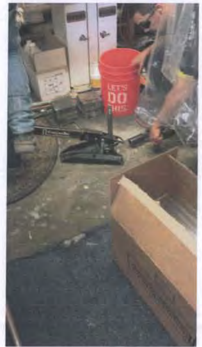
View of the had probe set-up used to drill boring B1E located near the pretreatment area.
