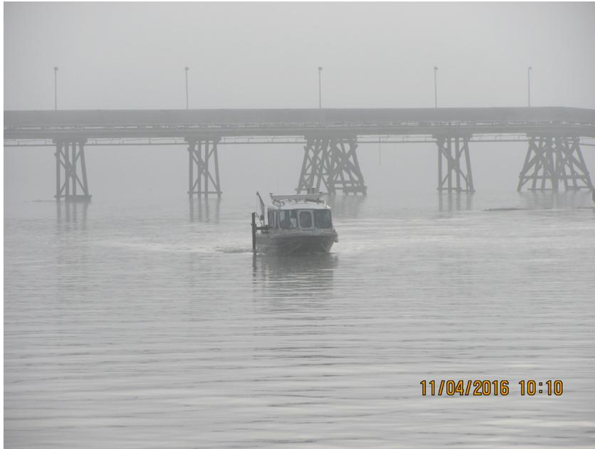
Multibeam hydrographic survey vessel running transects in the fog.
