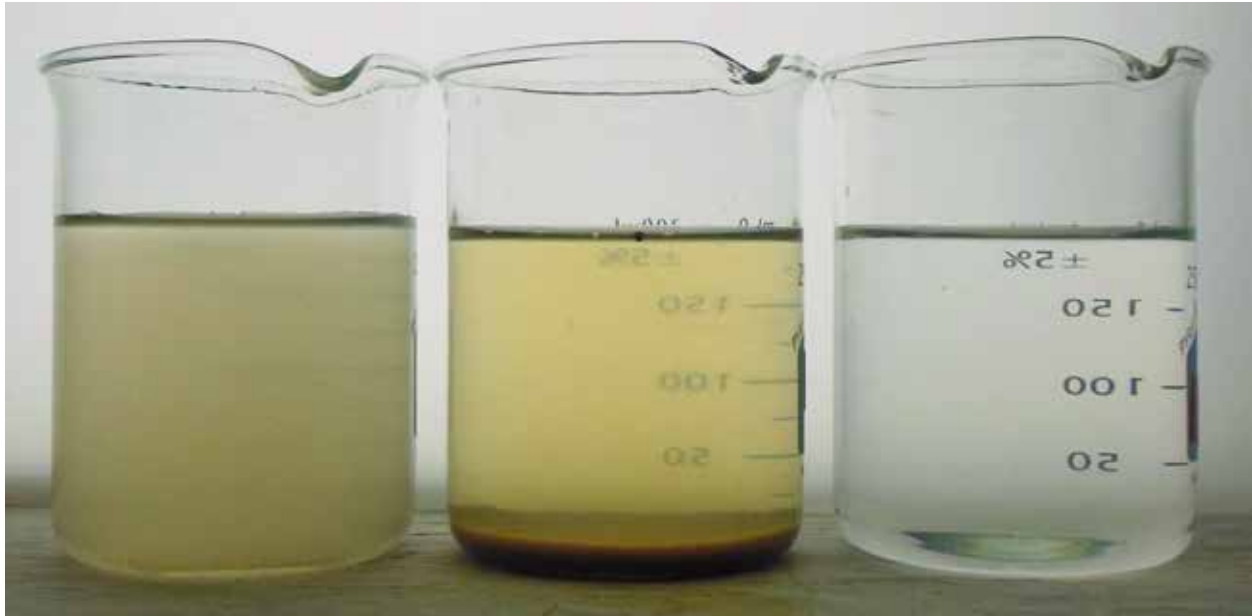
Figure 1 PERC - SLON; Influent (left), EC Effluent (center), Filtered EC Effluent (right).
