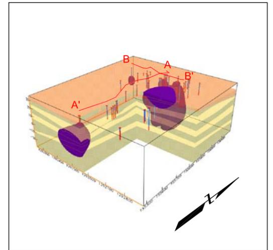
THREE-DIMENSIONAL ISOCONCENTRATION SHELL AT 50 ppb AND LOCATION OF CROSS-SECTION
