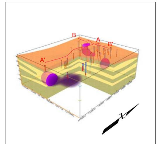
THREE-DIMENSIONAL ISOCONCENTRATION SHELL AT 1 ppb AND LOCATION OF CROSS-SECTION
