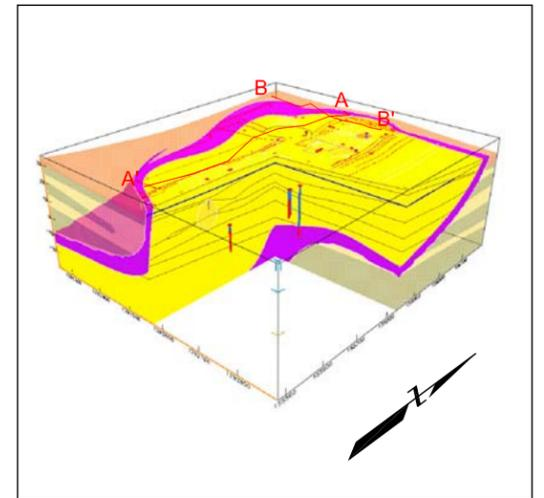
THREE-DIMENSIONAL ISOCONCENTRATION SHELL AT 0.5 ppb AND LOCATION OF CROSS-SECTION
