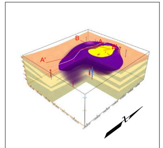
THREE-DIMENSIONAL ISOCONCENTRATION SHELL AT 500 ppb AND LOCATION OF CROSS-SECTION
