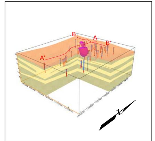
THREE-DIMENSIONAL ISOCONCENTRATION SHELL AT 0.11 ppb AND LOCATION OF CROSS-SECTION
