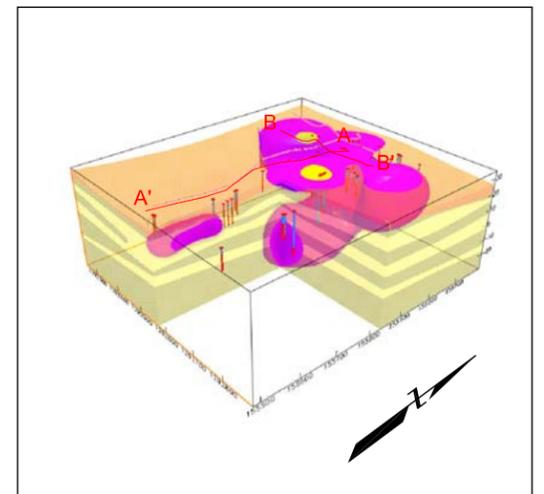
THREE-DIMENSIONAL ISOCONCENTRATION SHELL AT 10 ppb AND LOCATION OF CROSS-SECTION
