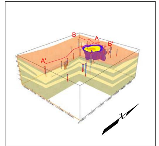
THREE-DIMENSIONAL ISOCONCENTRATION SHELL AT 800 ppb AND LOCATION OF CROSS-SECTION
