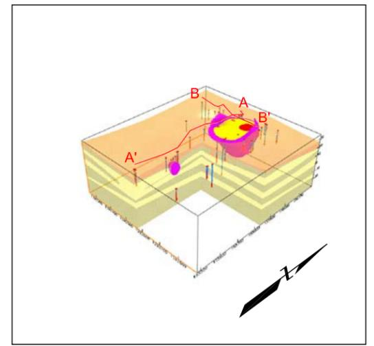
THREE-DIMENSIONAL ISOCONCENTRATION SHELL AT 0.795 ppb AND LOCATION OF CROSS-SECTION
