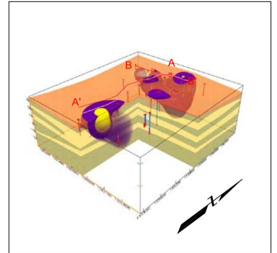
THREE-DIMENSIONAL ISOCONCENTRATION SHELL AT 0.54 ppb AND LOCATION OF CROSS-SECTION
