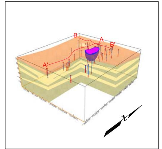
THREE-DIMENSIONAL ISOCONCENTRATION SHELL AT 0.025 ppb AND LOCATION OF CROSS-SECTION
