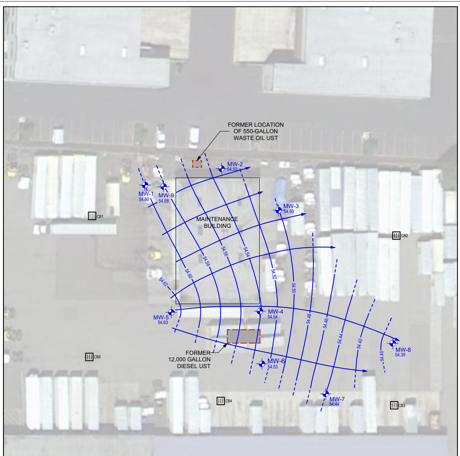
FIGURE 3 SEPTEMBER 5, 2017 GROUNDWATER ELEVATION CONTOURS AND FLOW DIRECTION
